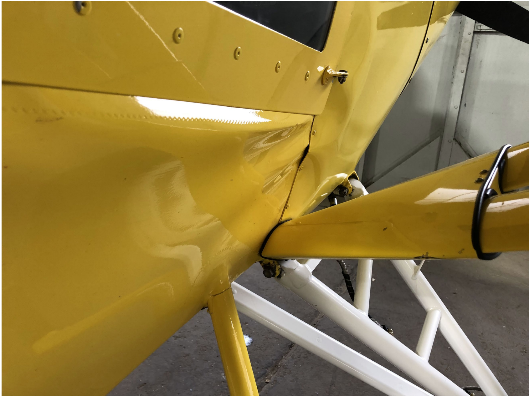
Accident Airplane / Gear Attach Point (Forward) / Fuselage – (Photo provided by the pilot)
