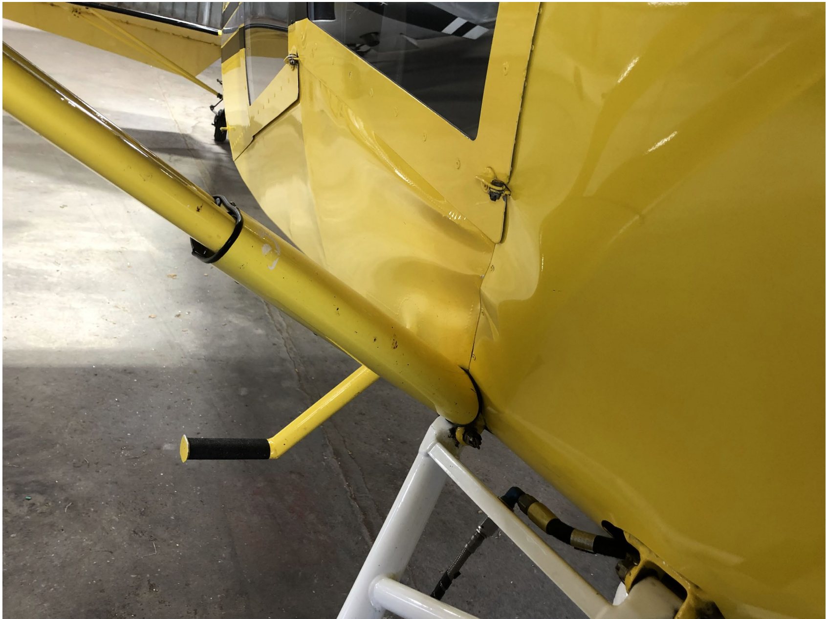
Accident Airplane / Gear Attach Point (Aft) / Fuselage – (Photo provided by the pilot)
