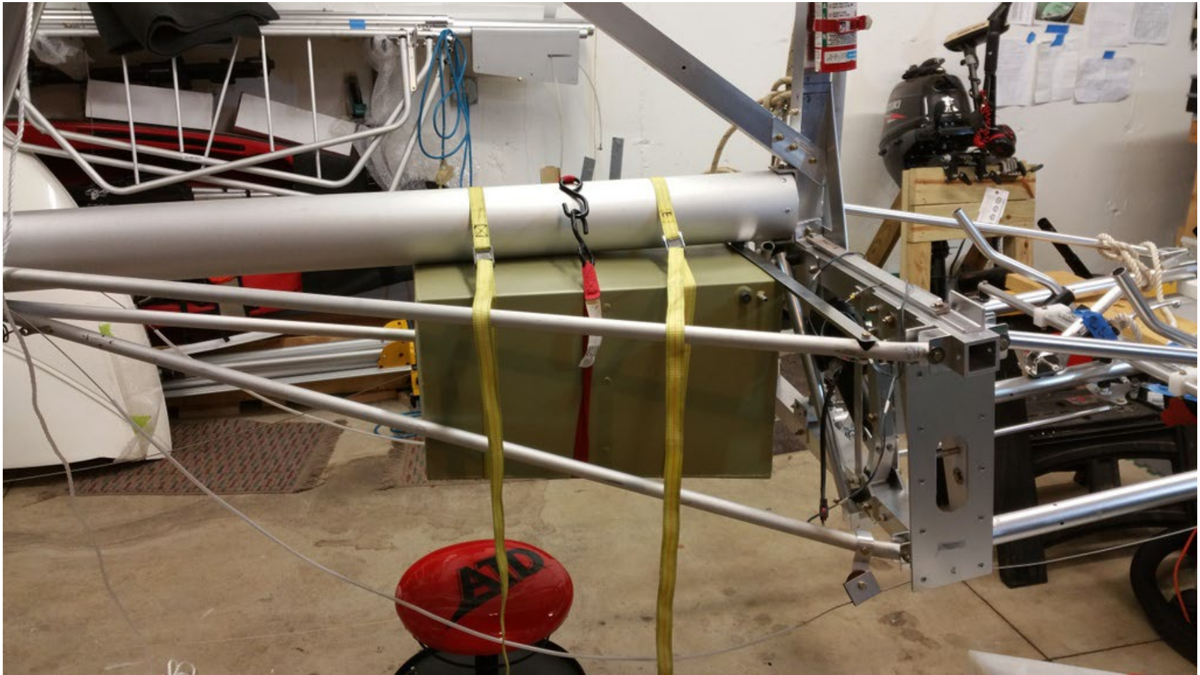
Exemplar Fuel Tank in a Similar Airplane (Courtesy of Federal Aviation Administration)
