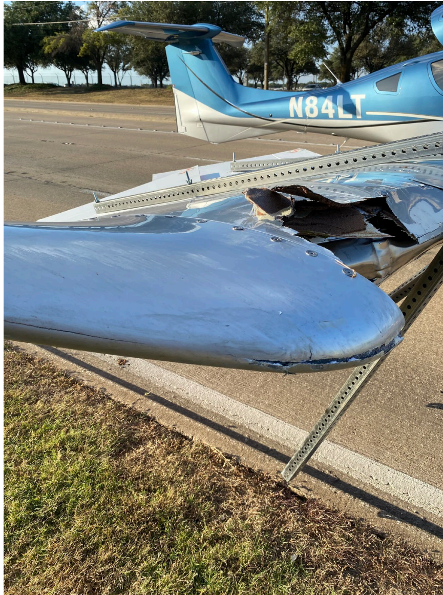
Photograph 2 - Right Wing Damage - Side View (Courtesy of FAA)
