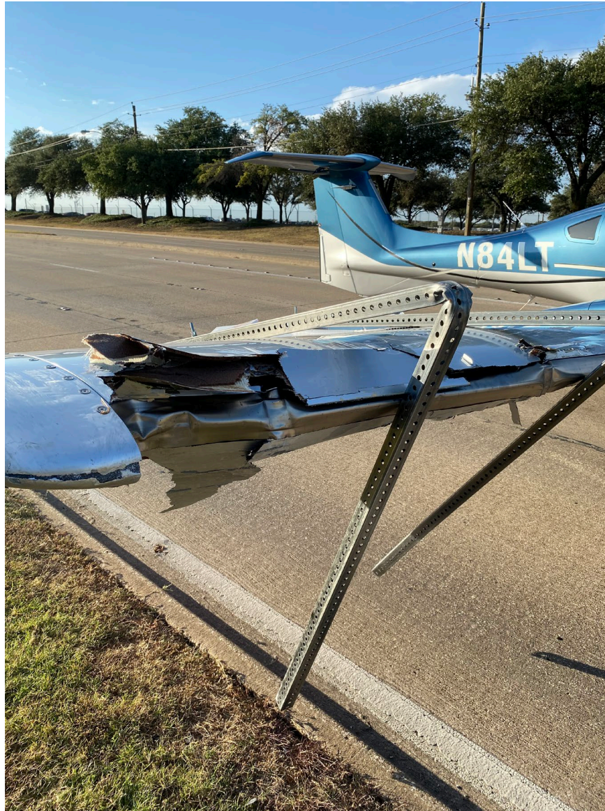
Photograph 1 - Right Wing Damage - Front View (Courtesy of FAA)
