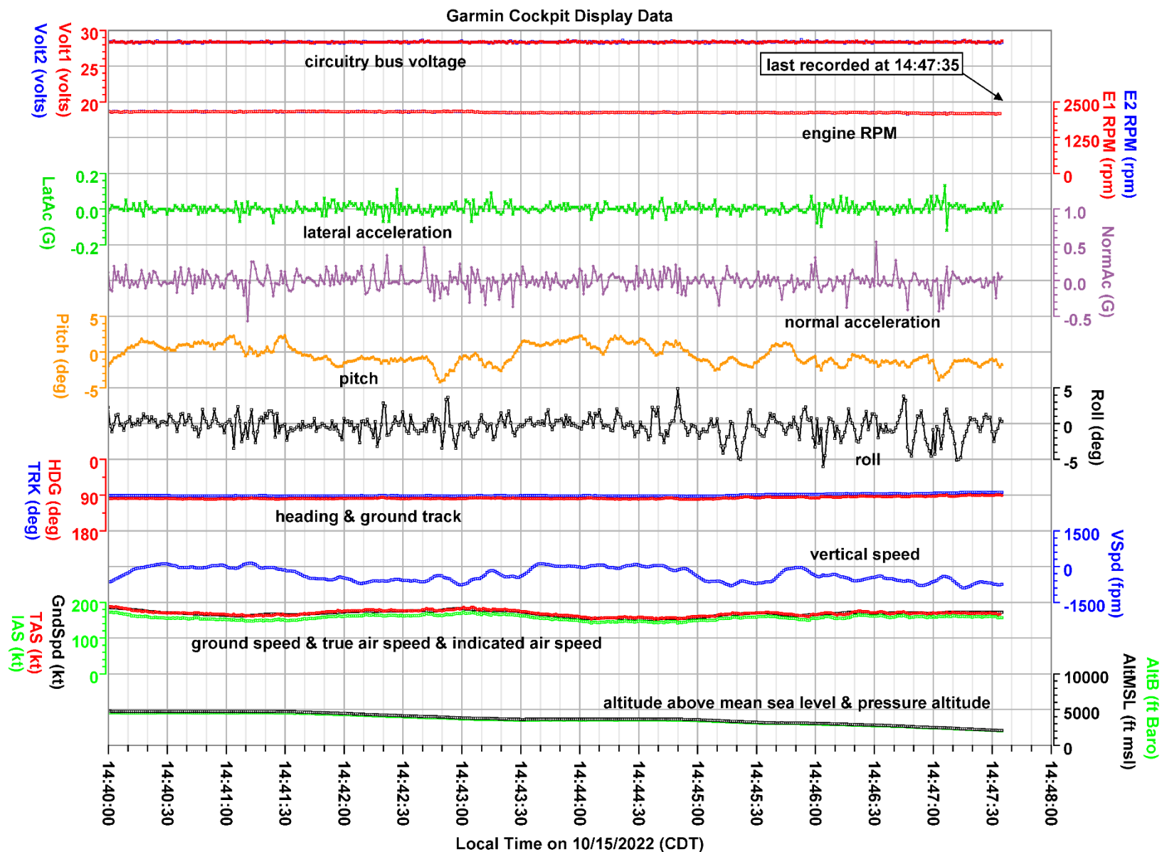
Figure 6. Plot of basic parameters of the Garmin cockpit display data for the end of the event flight.
