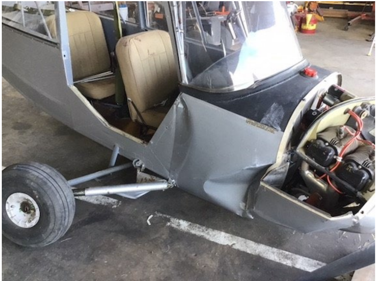
Photo 1: Fuselage Damage (Source – Federal Aviation Administration)
