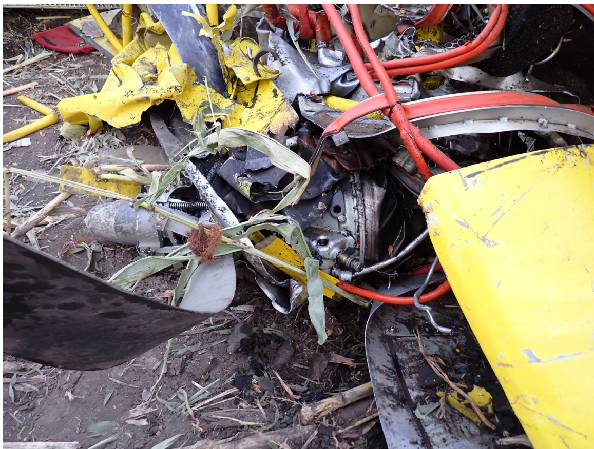
Photograph 6 - Torsional deformation noted to exhaust duct case (Courtesy of NTSB)
