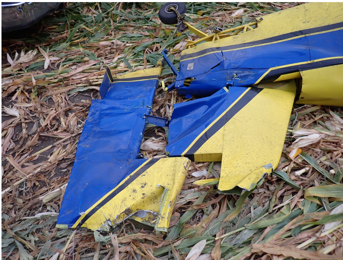
Photograph 2 - Impact damage and power line impressions (Courtesy of NTSB)
