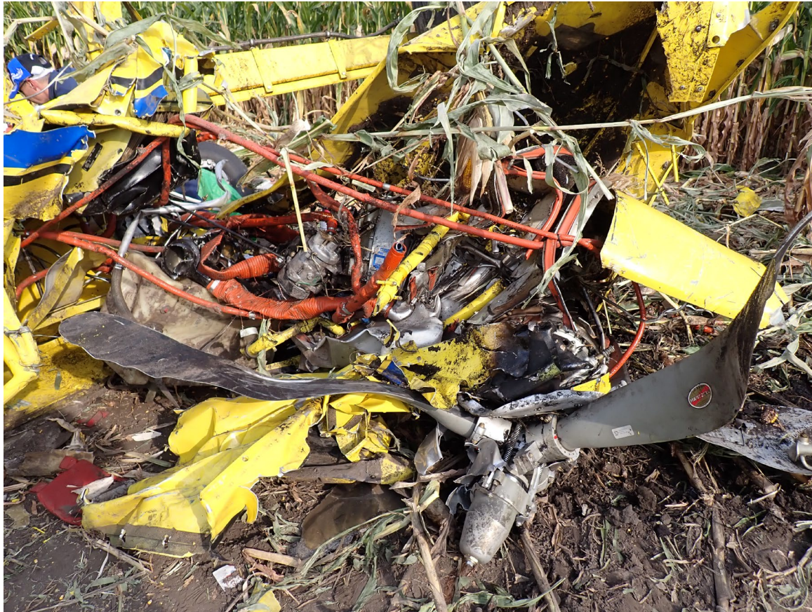
Photograph 5 - S-type bending noted to propeller blades (Courtesy of NTSB)
