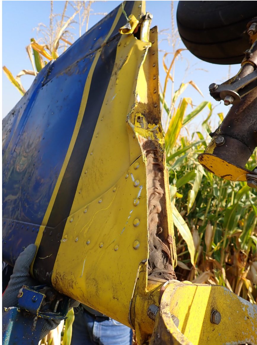
Photograph 4 - Deformation to bottom of rudder from tailwheel (Courtesy of NTSB)
