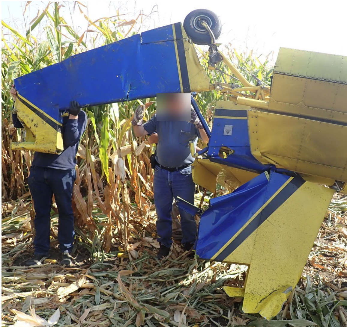
Photograph 3 - Deformation noted to bottom of rudder (Courtesy of Air Tractor)
