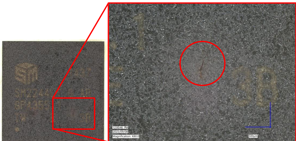
Figure 4. Microscope images of the SSD controller chip (left image) and zoomed in area showing overheating damage (right image).
