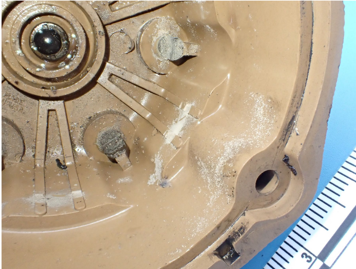
Photograph 3 - Ignition Distributor cap with scoring (NTSB Photo)
