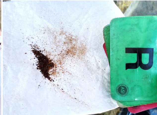
Figure 11. Debris from right fuel line
