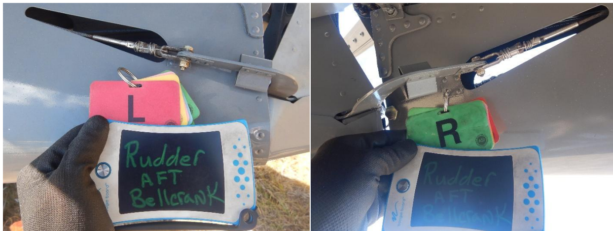
Figure 3. Postaccident rudder bellcrank connections (left and right)
