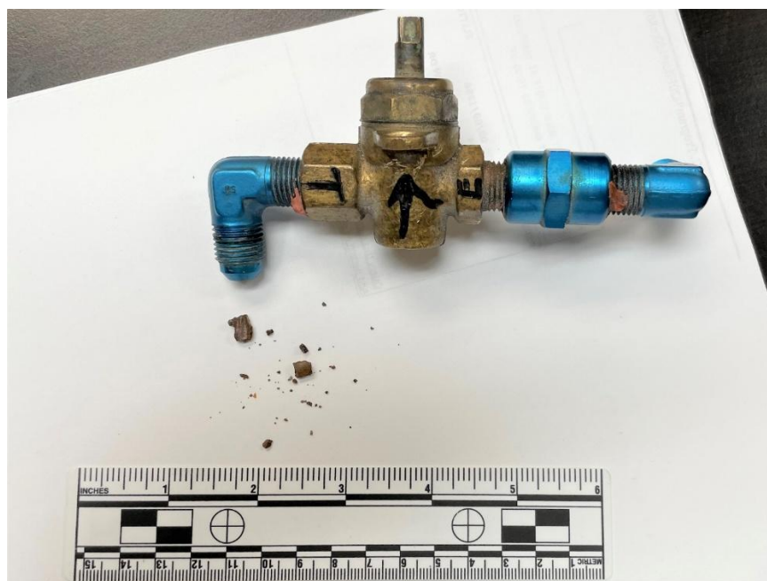
Figure 9. Fuel shutoff valve with debris from inlet port
