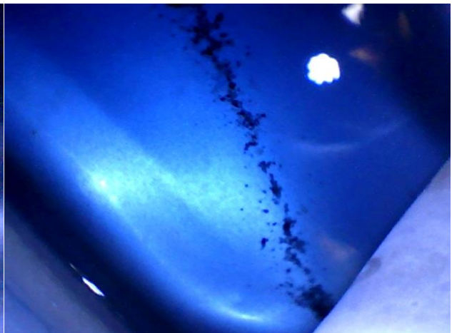
Figure 13. Debris in right fuel tank
