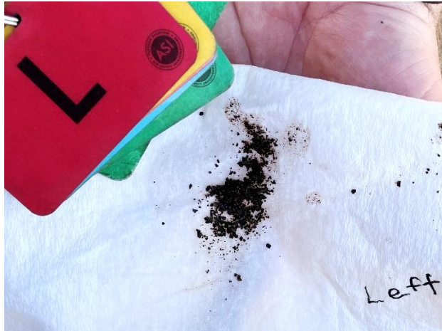
Figure 10. Debris from left fuel line
