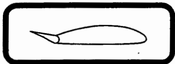
Flap in speed flight setting
