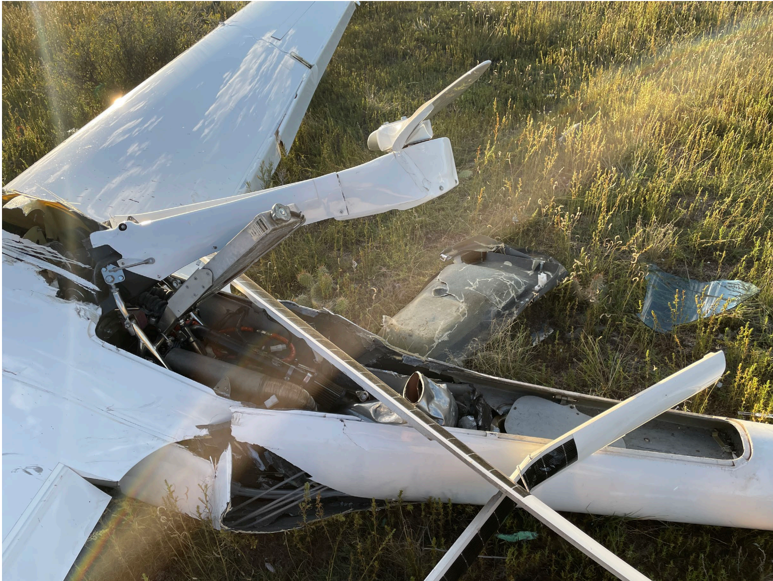
Photograph 2 - Empennage, Retractable Propeller and Engine Radiator
