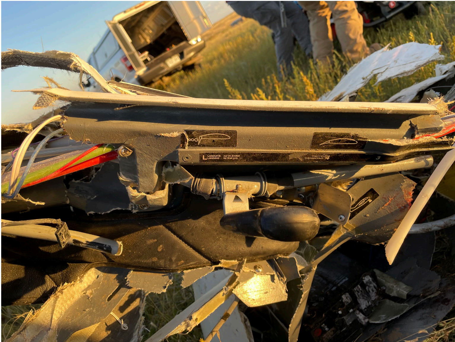
Photograph 7 - Flap Lever in Landing Position
