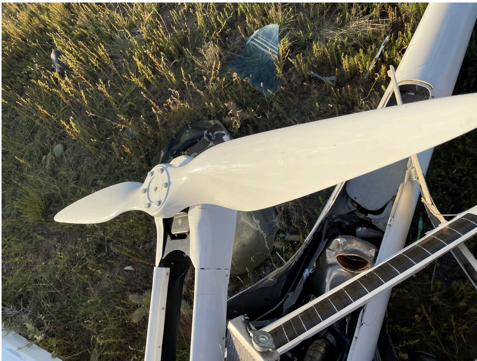
Photograph 3 - Propeller in Nonstandard Position
