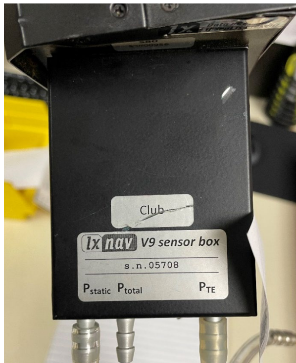
Figure 2. LXNAV V9 Sensor Box attached to S80 as received by Vehicle Recorder's Lab.
