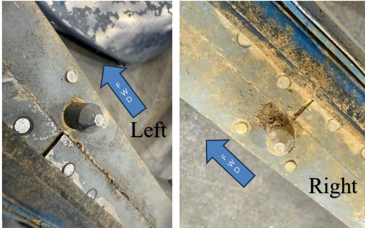
Figure 8. Guide pins (photos provided by Van's Aircraft)
