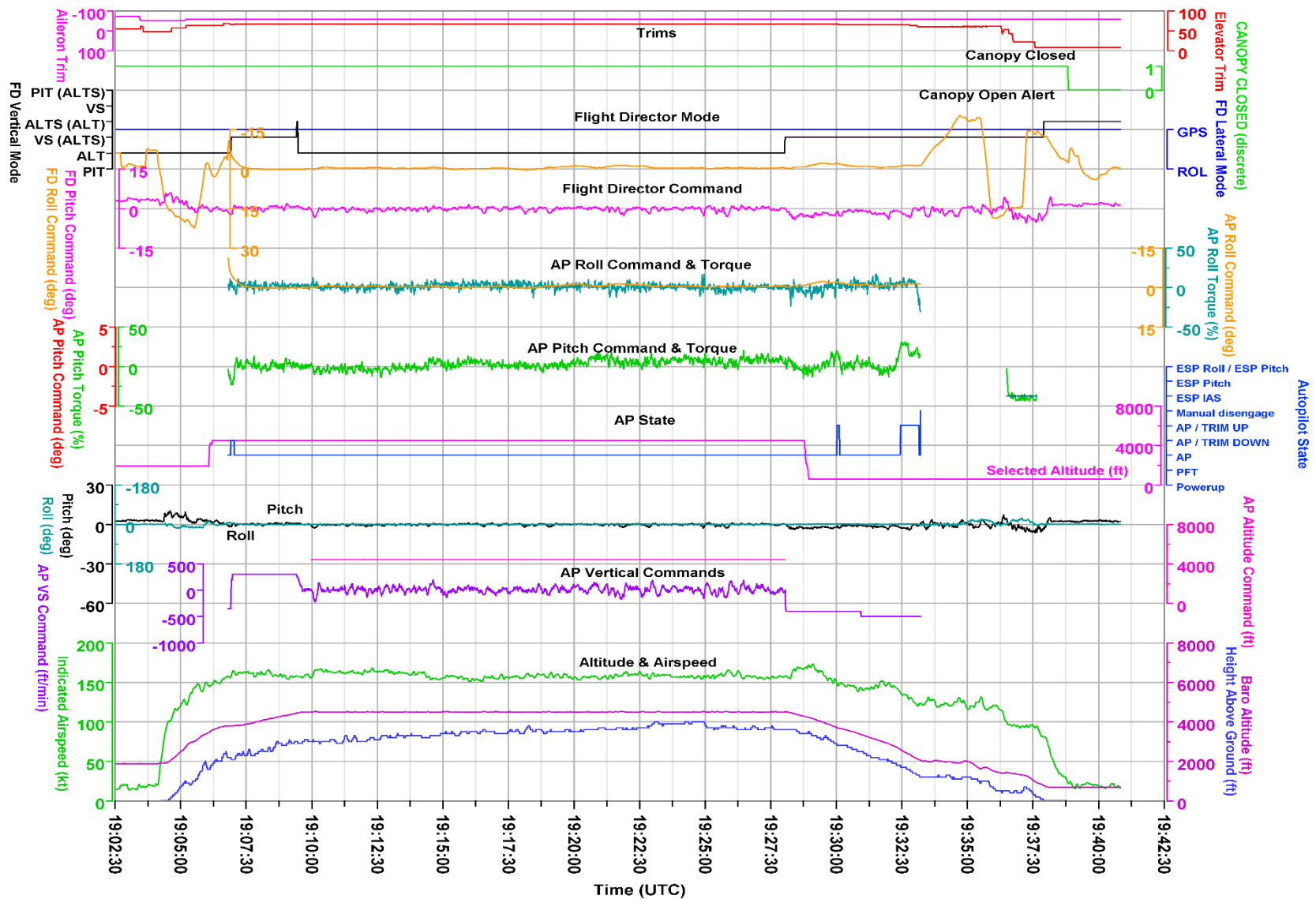
Figure 16. A plot of autopilot parameters during flight 37 which was conducted on June 17, 2023, showing the fifth leg of the flight.
