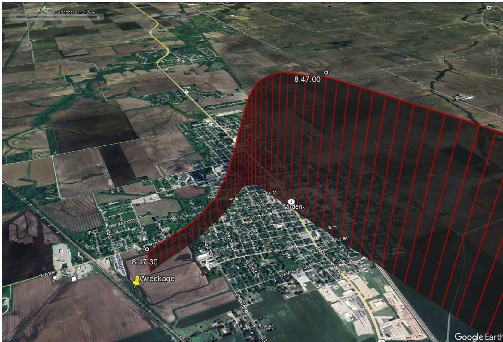
Figure 37. A Google Earth KML showing the aircraft's descent to the wreckage site. Note, the recorded altitude used to construct this KML may not accurately represent the aircraft's height above ground.
