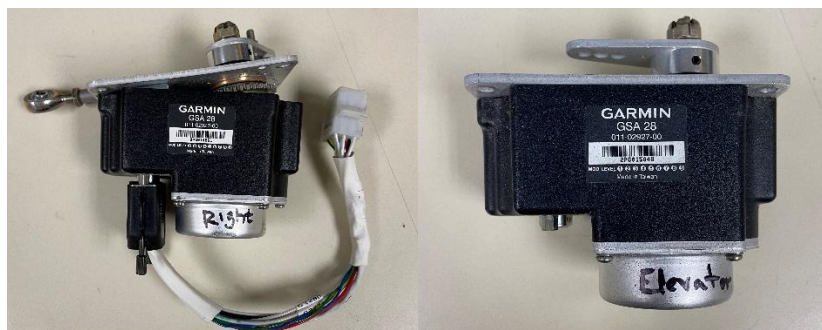
Figure 8. The roll servo recovered (left) and the pitch servo (right). Note that the servos had been removed by the salvager, and the condition is not necessarily representative of the installed state.
