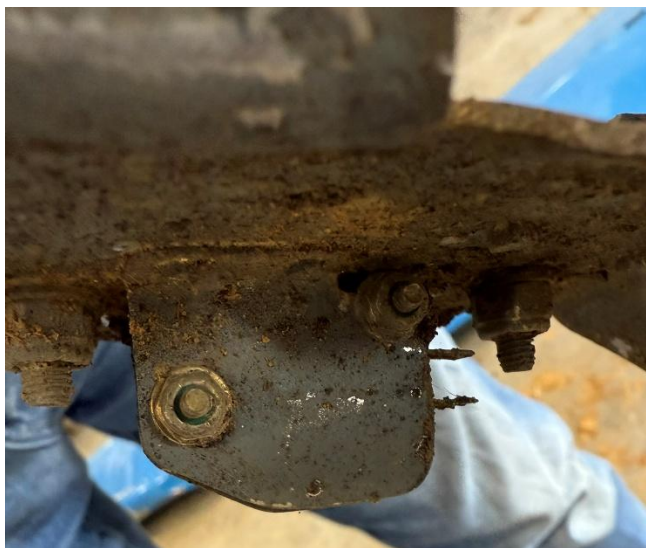
Figure 3. The canopy latch micro switch as recovered, installed in the location defined in the aircraft's plans.
