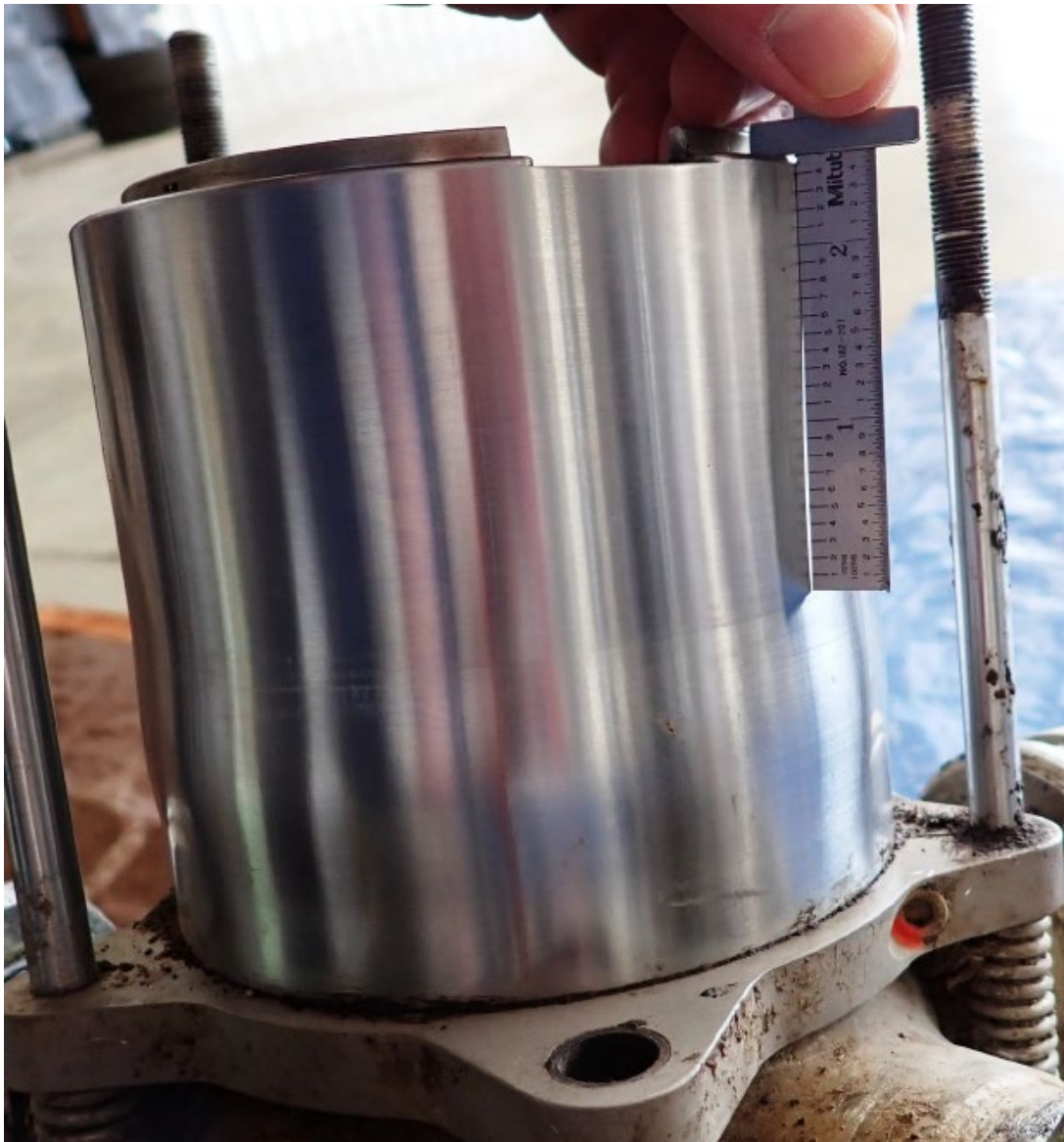
Figure 3. Cylinder bulge at 2.5" below top corner
