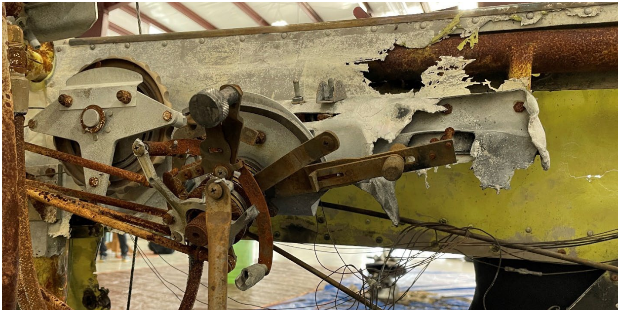
Figure 7. The power quadrant lever positions during the examination.
