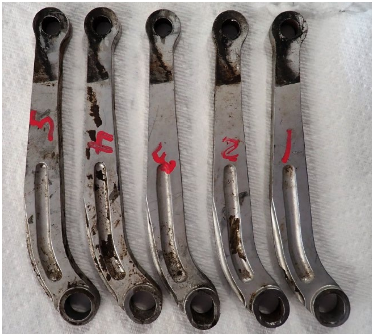
Figure 4. Link arm comparison showing stretch on No. 1-4
