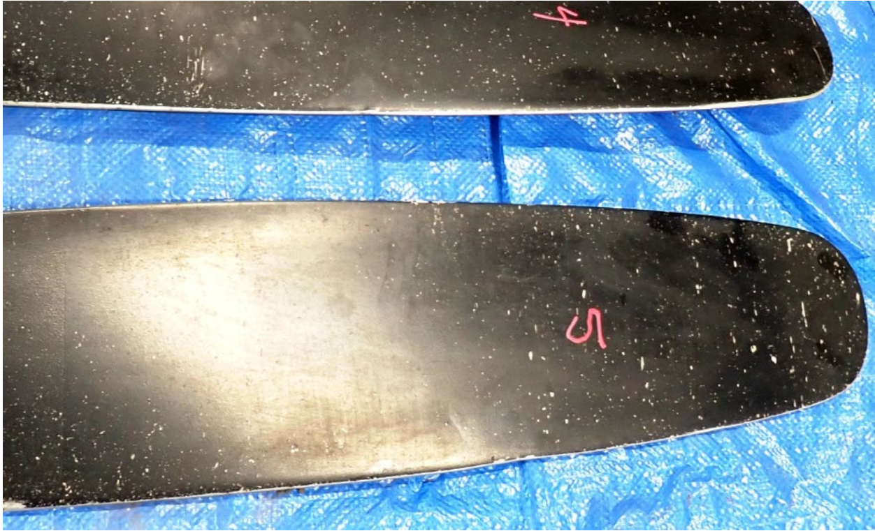
Figure 5. Light, face-side abrasion on blade No. 5, similar on all blades
