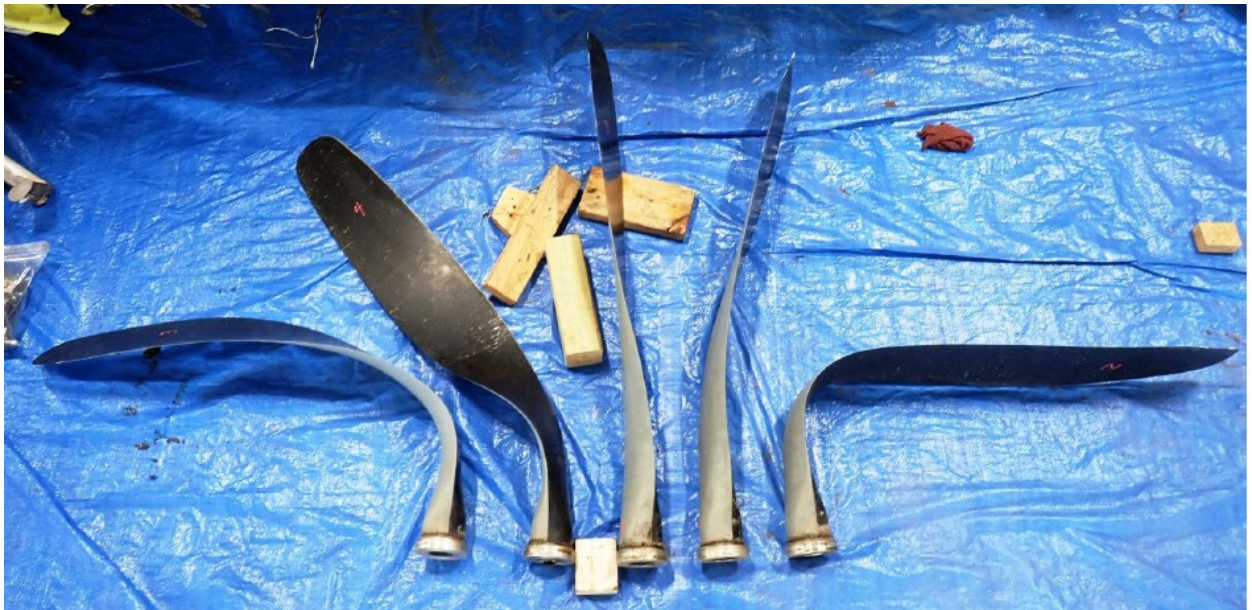
Figure 6. Propeller blades trailing edge view 3-4-5-1-2 left-to-right.
