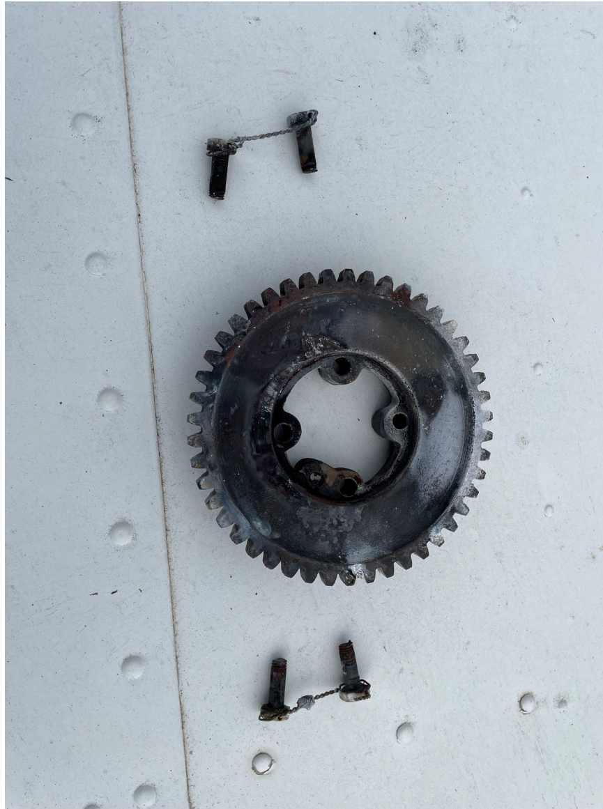
Photograph 6 - Crankshaft gear after removal from engine at accident site (NTSB Photo)
