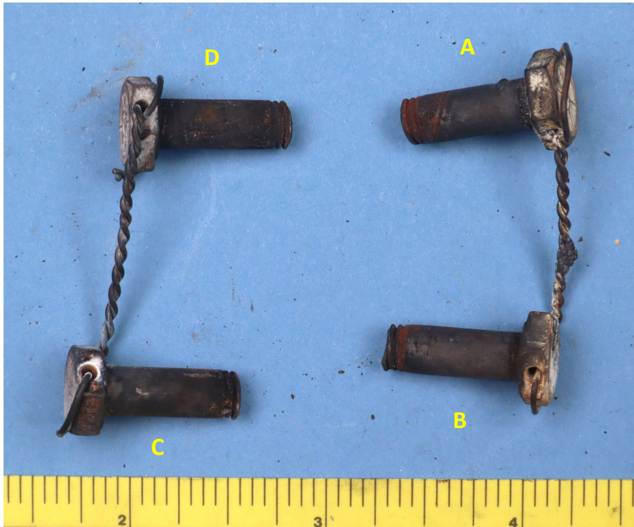
Figure 5. Macro photo of the fractured attachment bolts.
