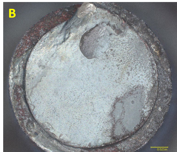
Figure 7. Digital microscope images of the fracture surfaces on the attachment bolts after cleaning.
