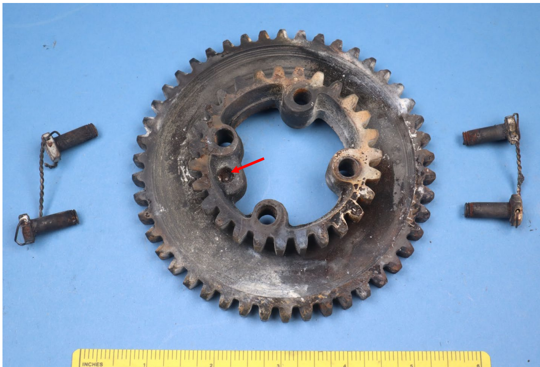
Figure 1. Macro photos of the submitted crankshaft gear and attachment bolts. The red arrows points to the dowel pin still assembled inside the gear.
