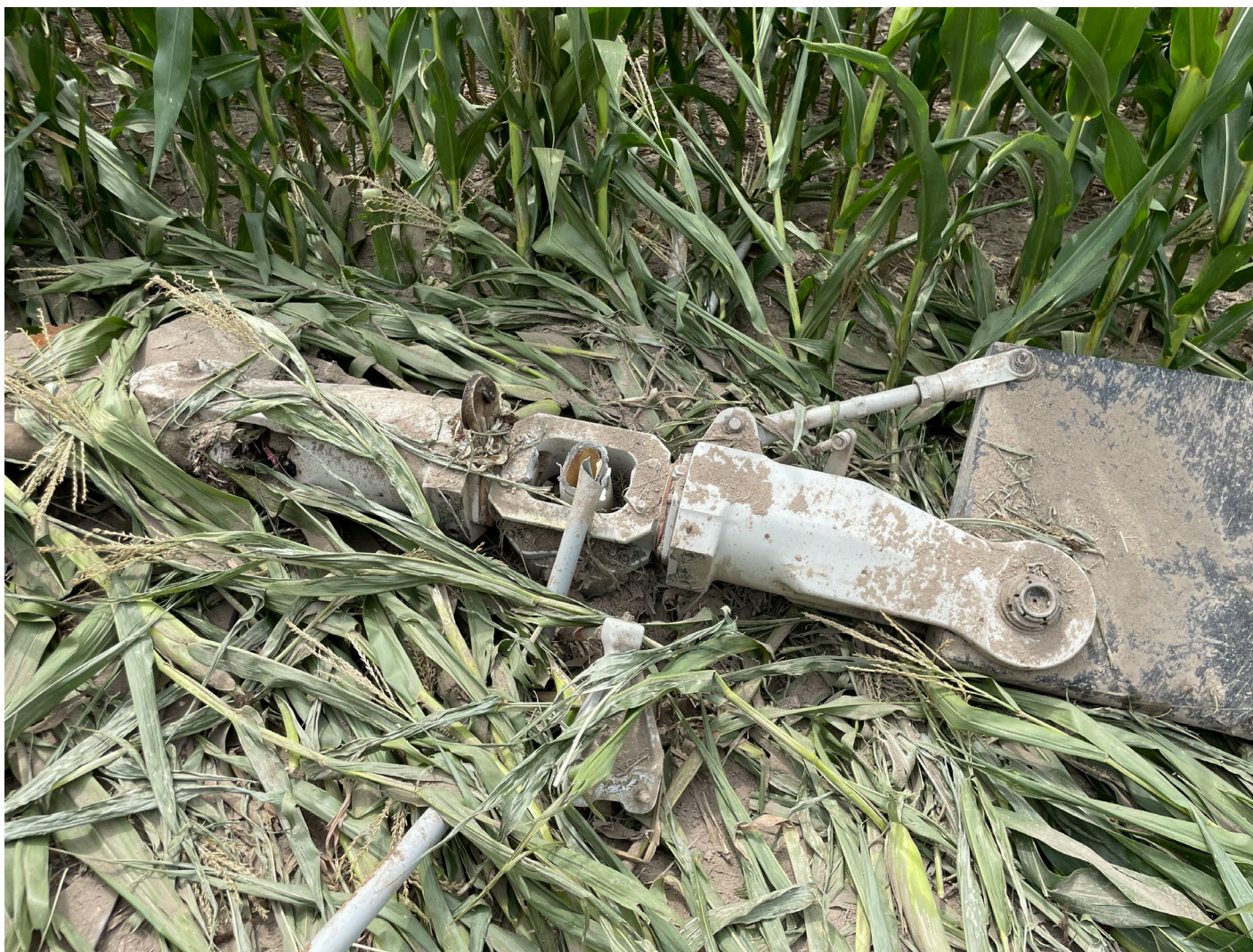
Photograph 2 - Main Rotor Hub
