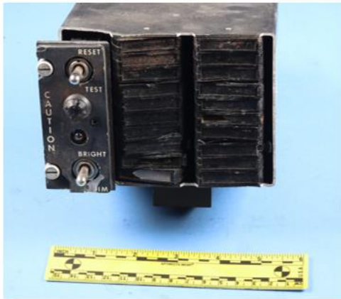
Figure 14. The caution panel as recovered from the cockpit instrument panel and a diagram of the typical caution panel layout.
