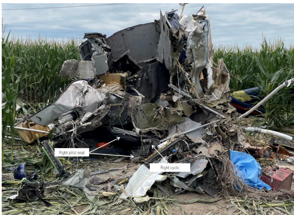
Figure 3. Wreckage view of the cockpit area with the right pilot seat and right cyclic stick identified.
