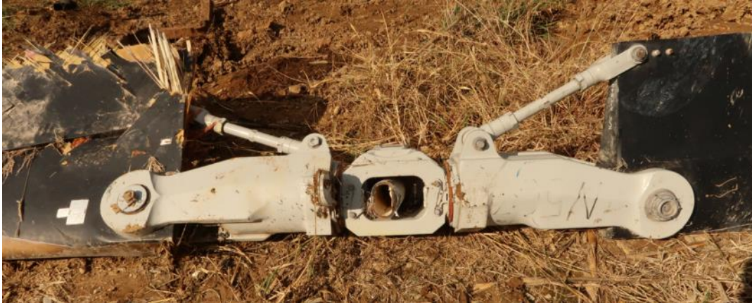
Figure 11. Rotor head had separated from the mast. Centered in the rotor head is a portion of the mast that had deformed into an oval shape.
