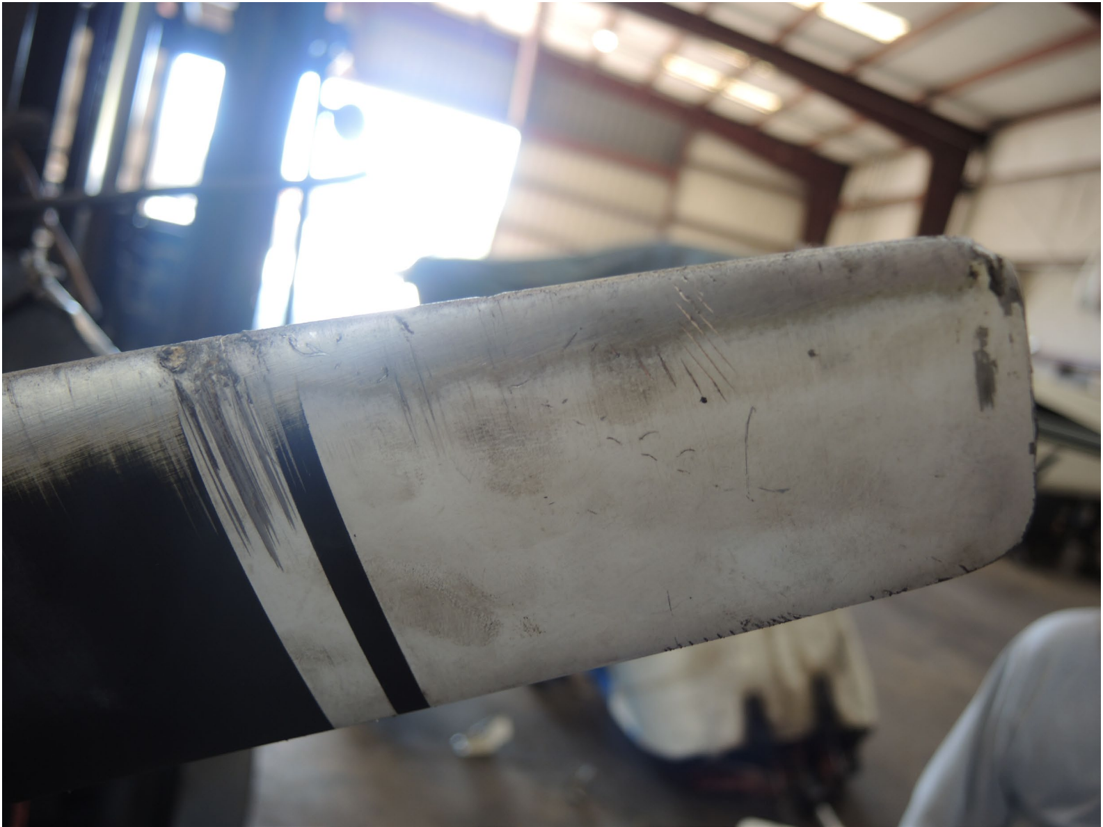
Photograph 19 - Propeller blade 2 damage
