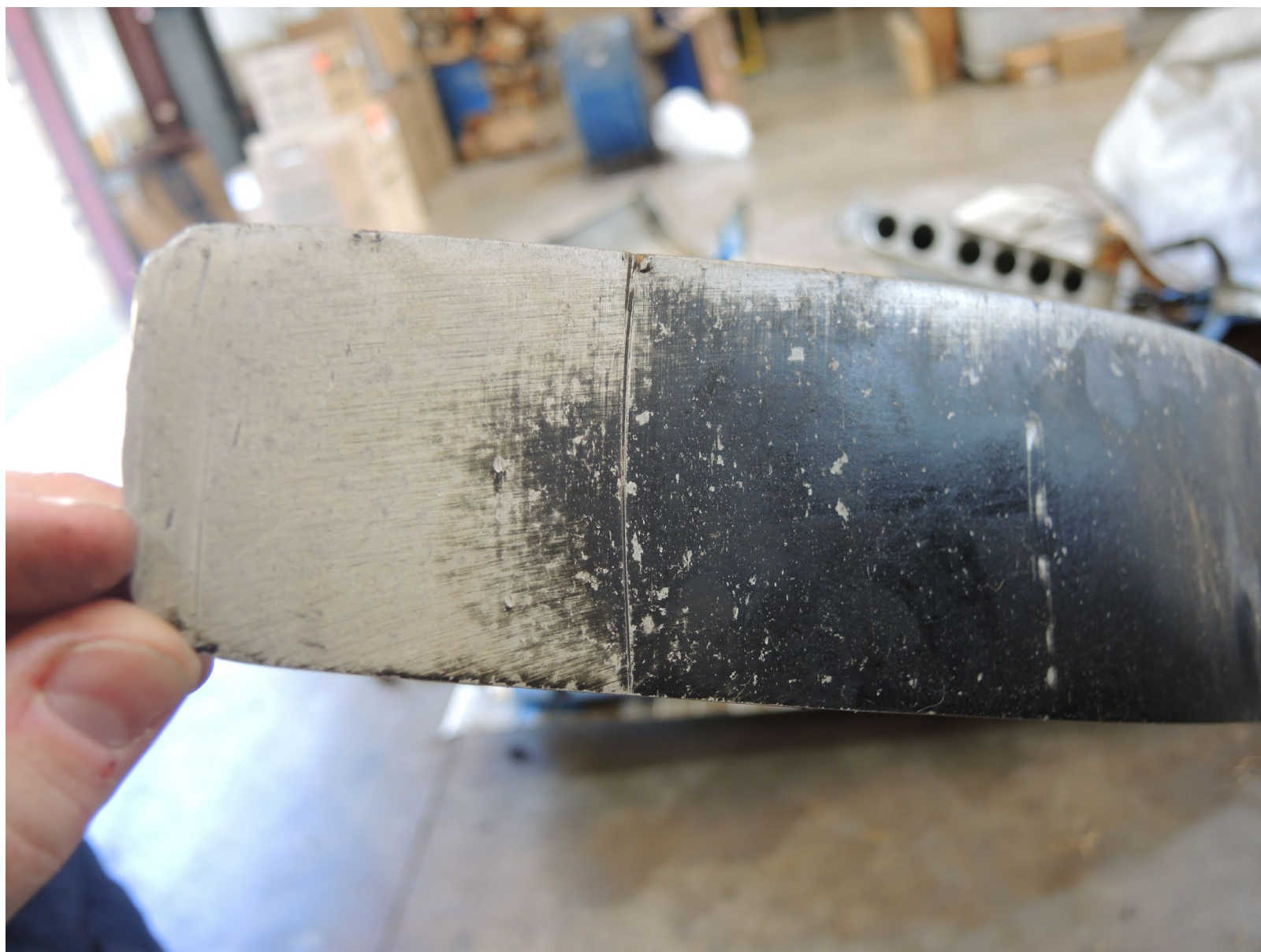
Photograph 18 - Propeller blade 2 damage, cambered side
