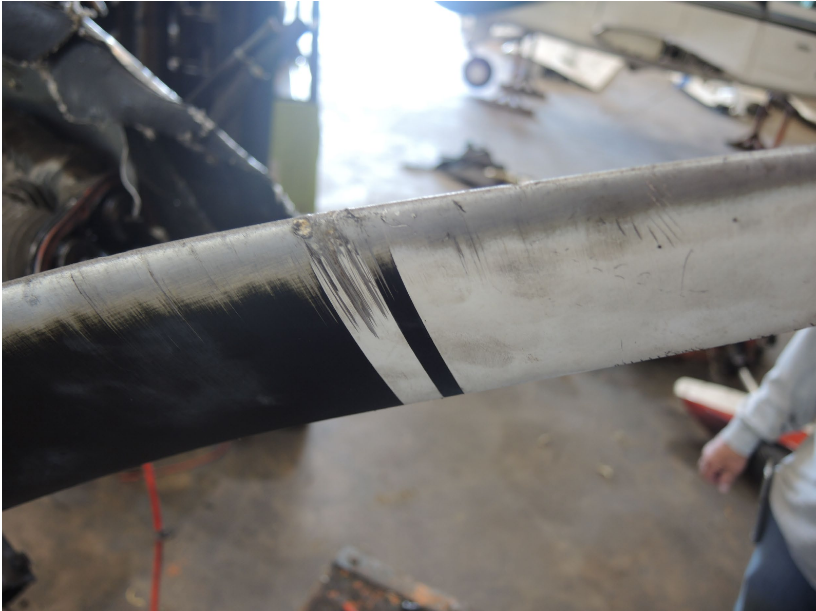
Photograph 17 - Propeller blade 2 damage
