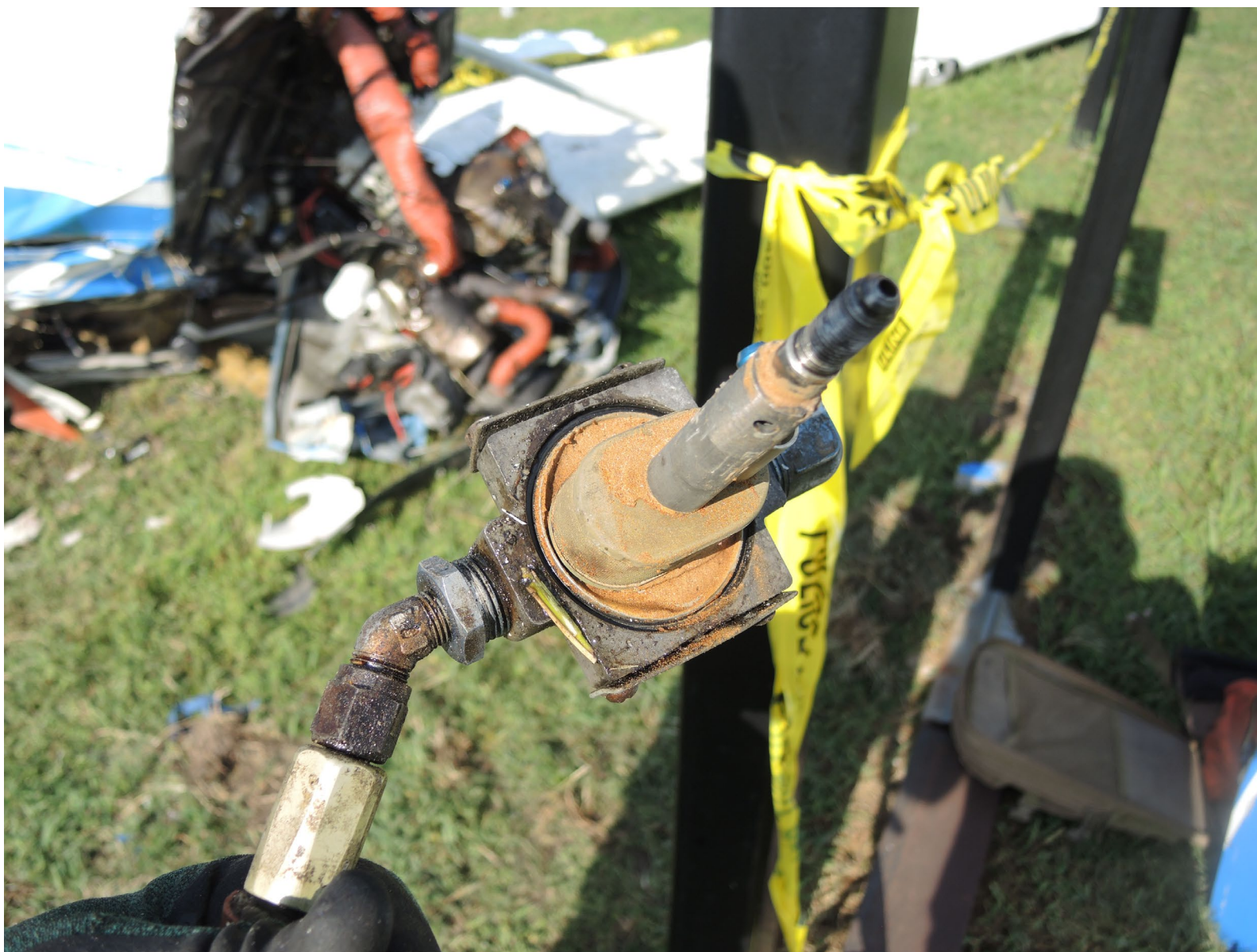
Photograph 9 - Debris in fuel strainer
