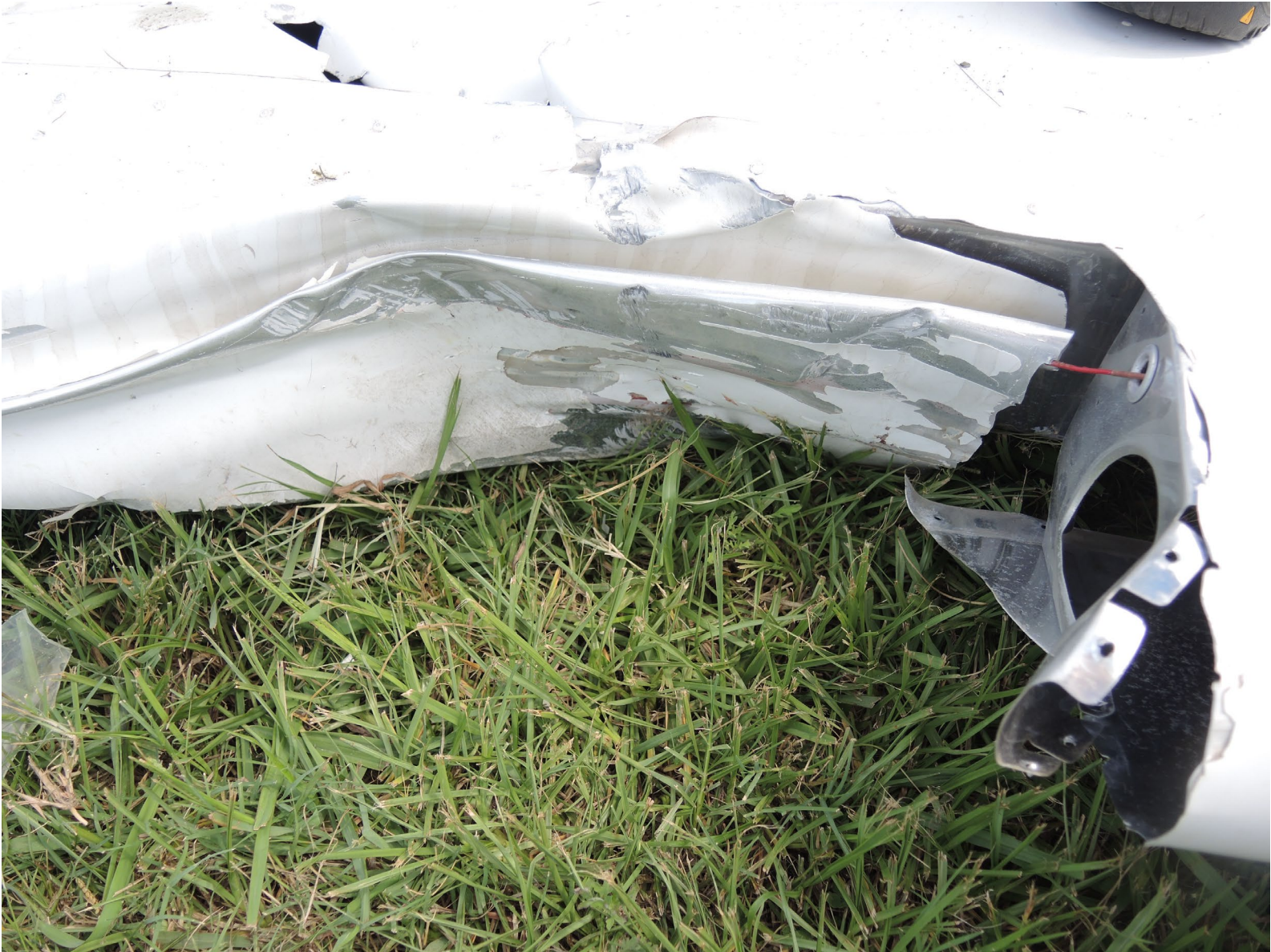
Photograph 8 - Right wing leading edge damage
