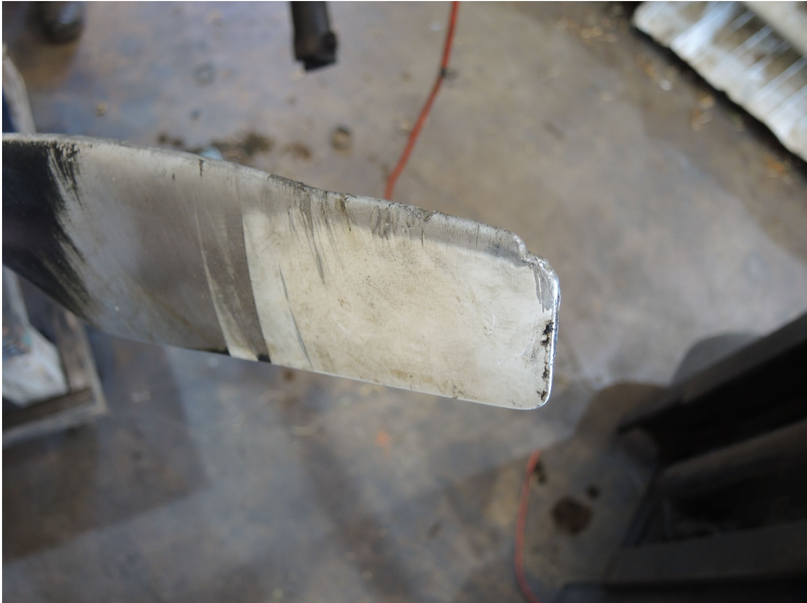
Photograph 16 - Propeller blade 1 damage
