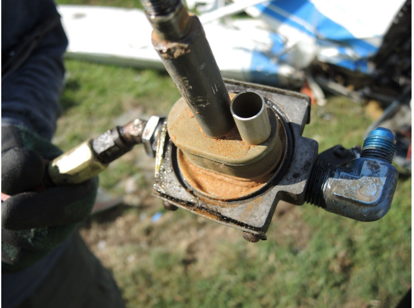
ASI-23-BT-115 (fuel strainer screen) (powder that lined fuel system)
