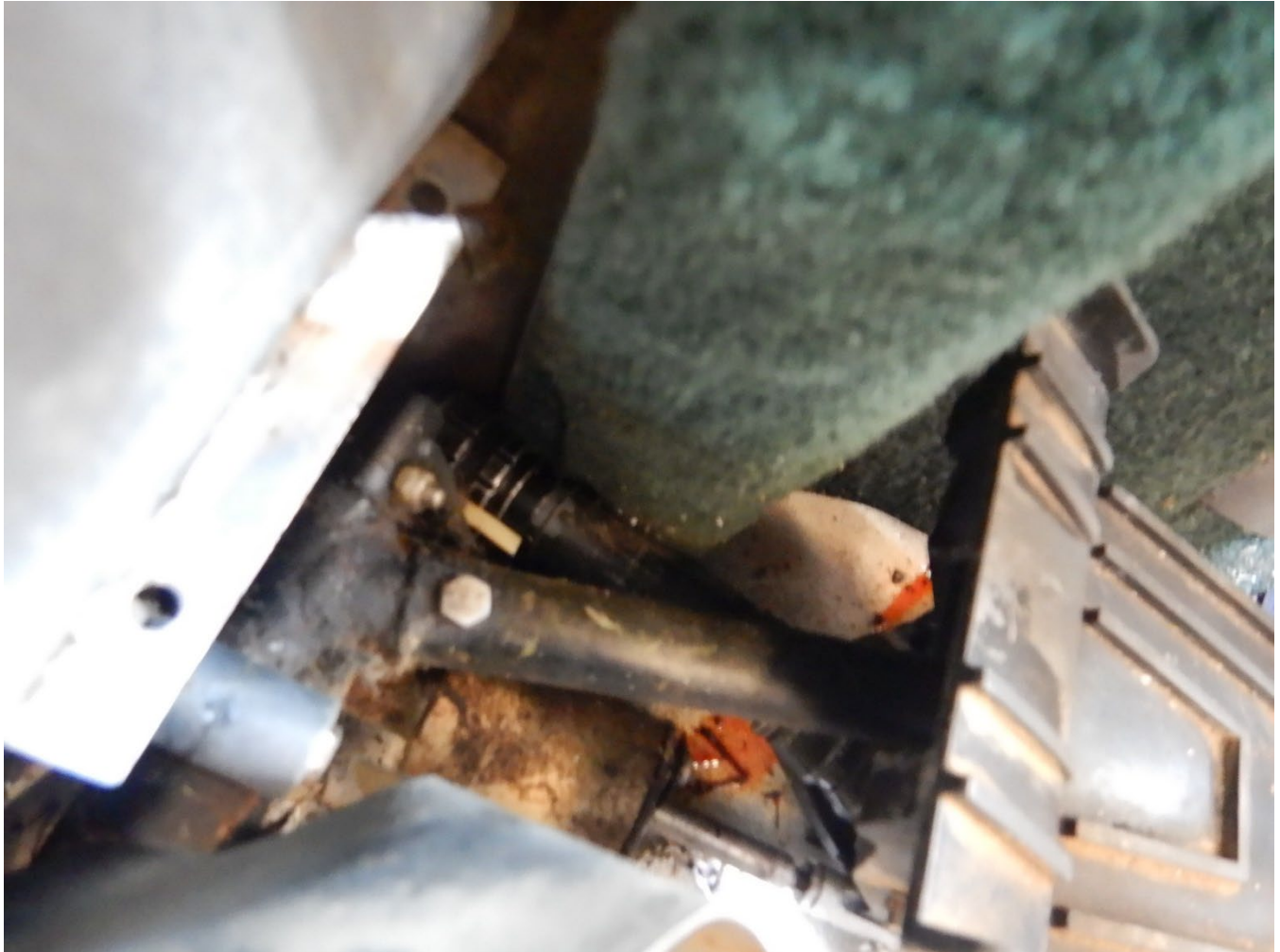
TAI Examination ASI-23-BT-030 (flashlight in rudder pedal)
