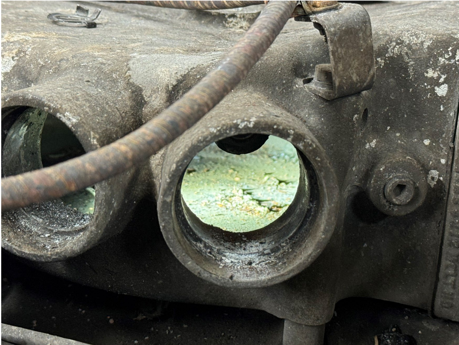
Photograph 10 - Right Engine Induction Housing Assembly Debris
