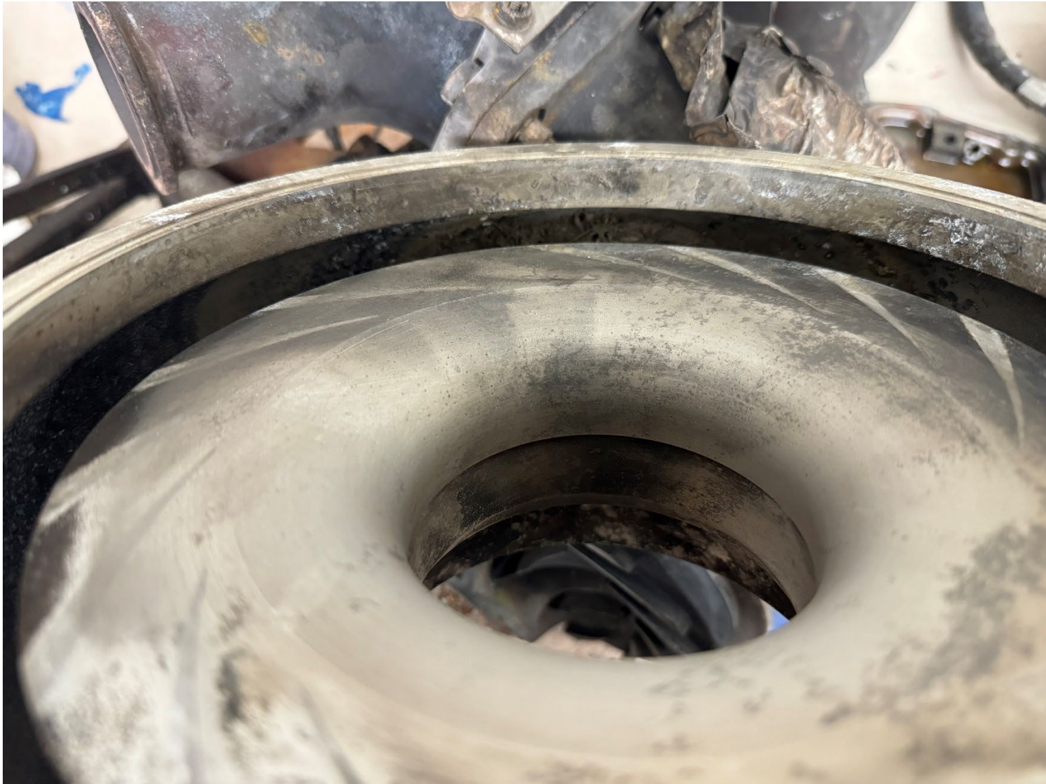
Photograph 9 - Right Engine Turbocharger Compressor Section
