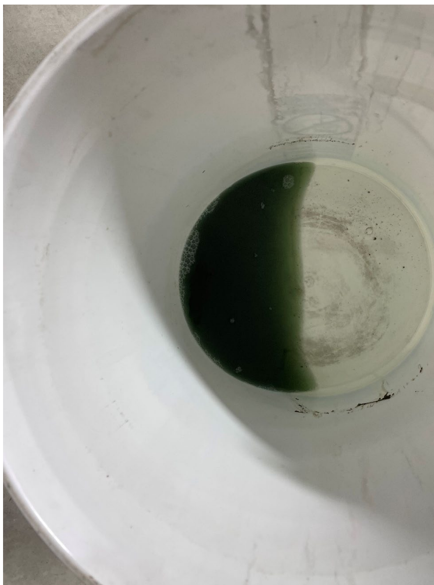
Photograph 12 - Preaccident Drained Fuel
