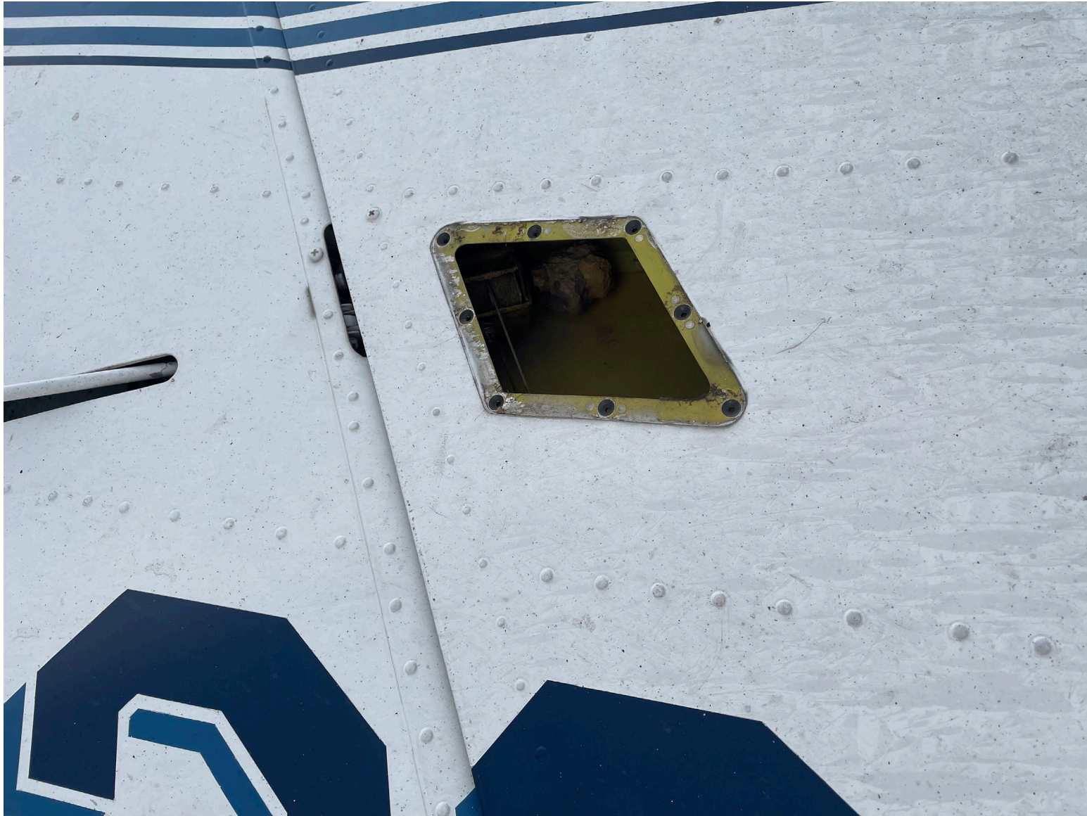
Photograph 6 - Preaccident Insect Nest around Elevator Trim Jackscrew
