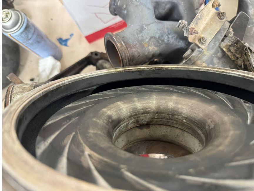
Figure 6. Compressor housing with rotational witness marks
