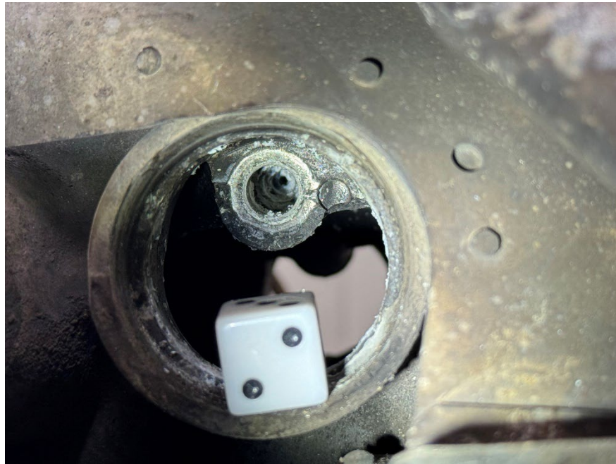
Figure 5. Example of the corrosion in the #2 Fuel Injector port.
