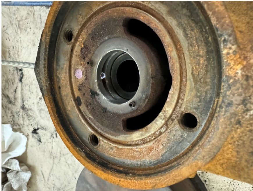
Figure 10. Turbocharger bearing and bearing oil gallery.
