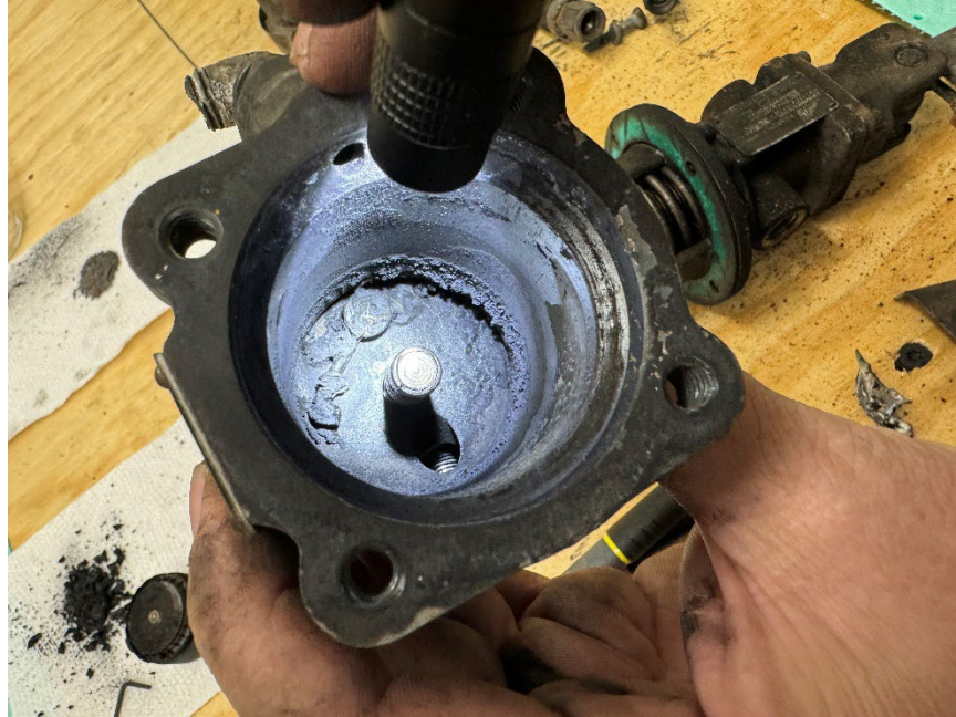
Figure 8. Wastegate Controller Housing (Oil Inlet Side)
