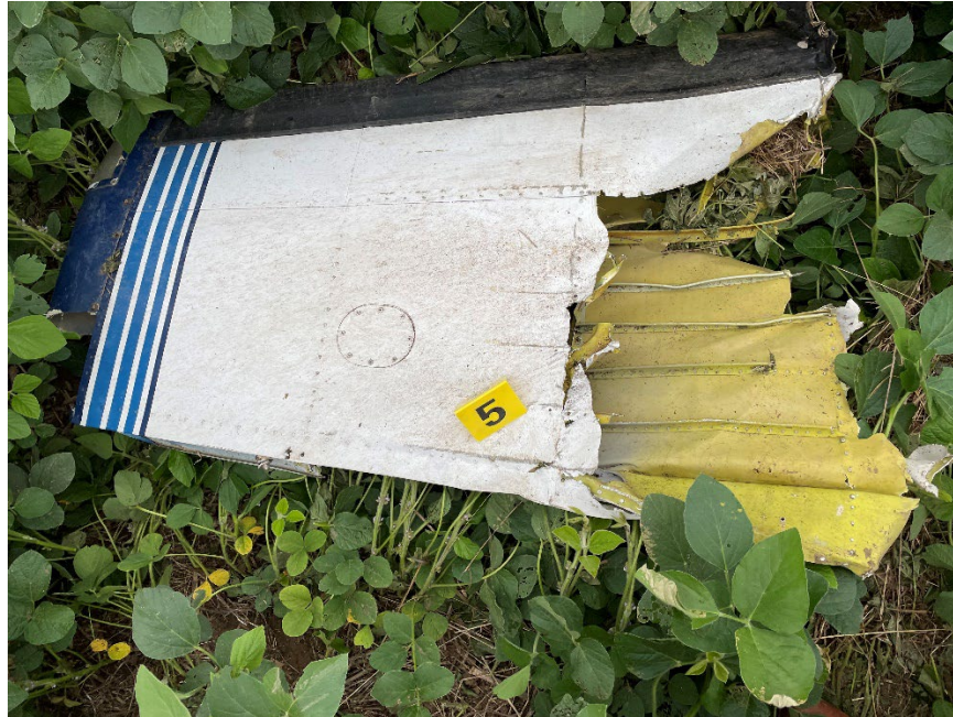
Figure 4: Separated outboard section of right wing
