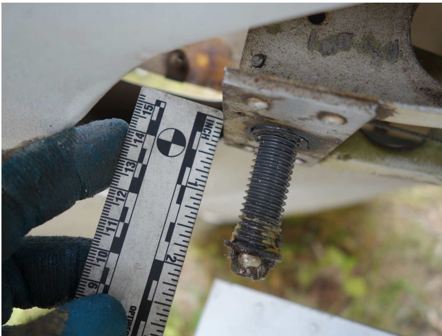
Photograph 12 - View of the trim tab jackscrew, with a ruler for measurement purposes, after it was recovered from the accident site (courtesy of Piper Aircraft).
