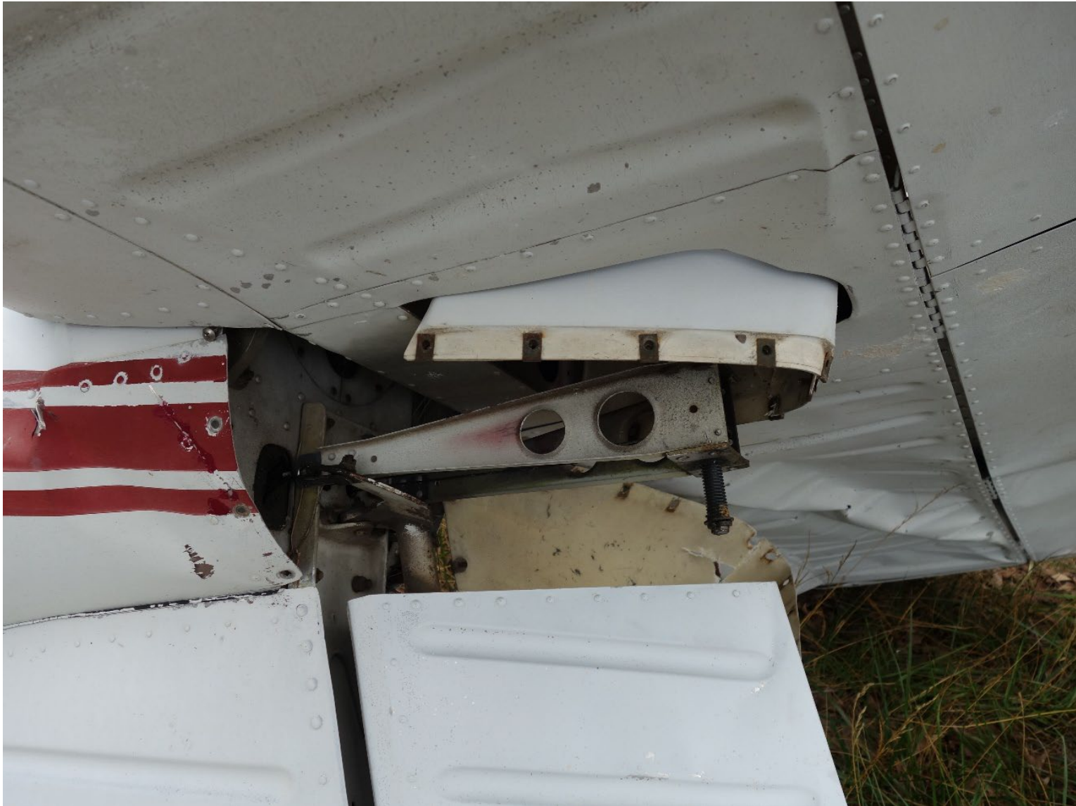
Photograph 11 - View of the trim tab jackscrew after it was recovered from the accident site (courtesy of Piper Aircraft).
