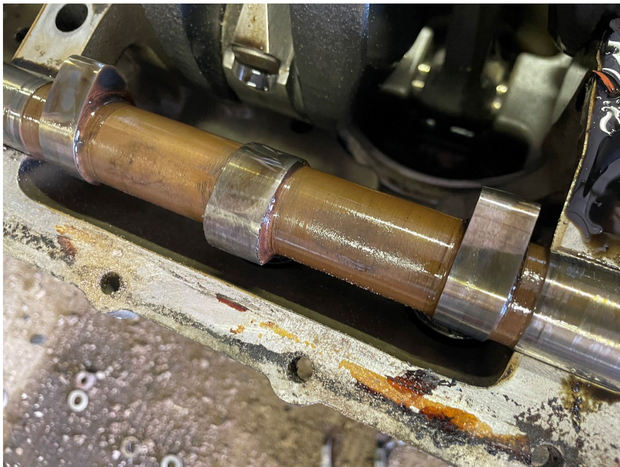
Figure 1 - Left engine Cylinder 3 & 4 Intake Lobe Spalling
