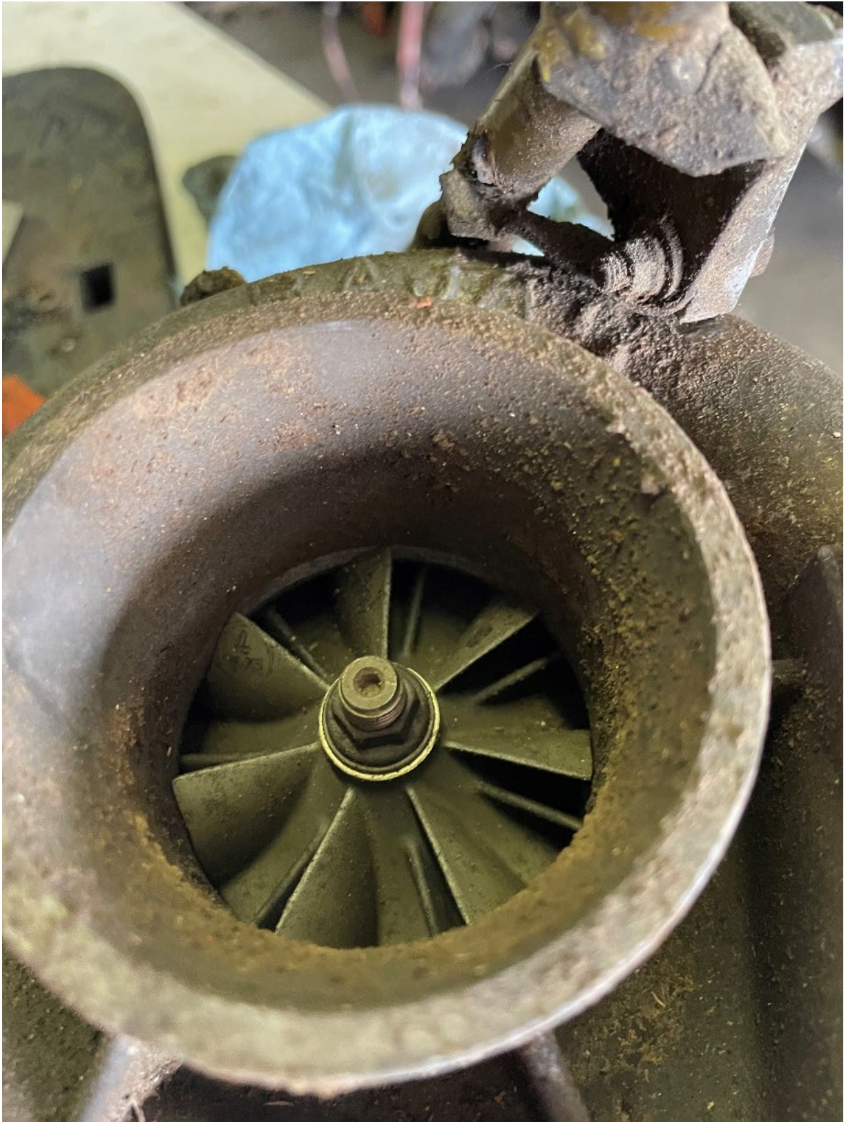
Figure 2 - Left Engine, Left Turbo Rotational Scoring
