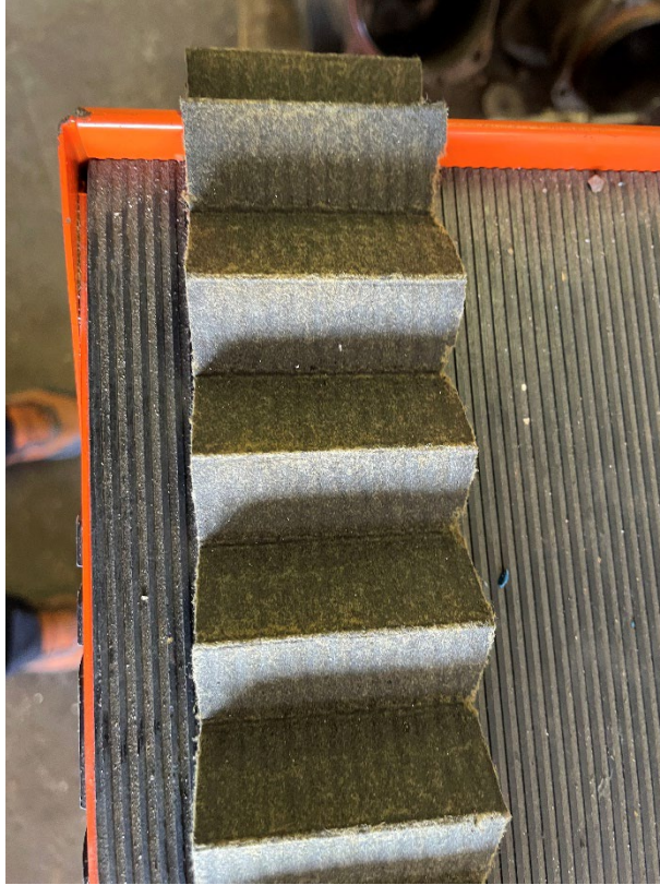
Figure 3 - Left Engine Oil Filter Media
