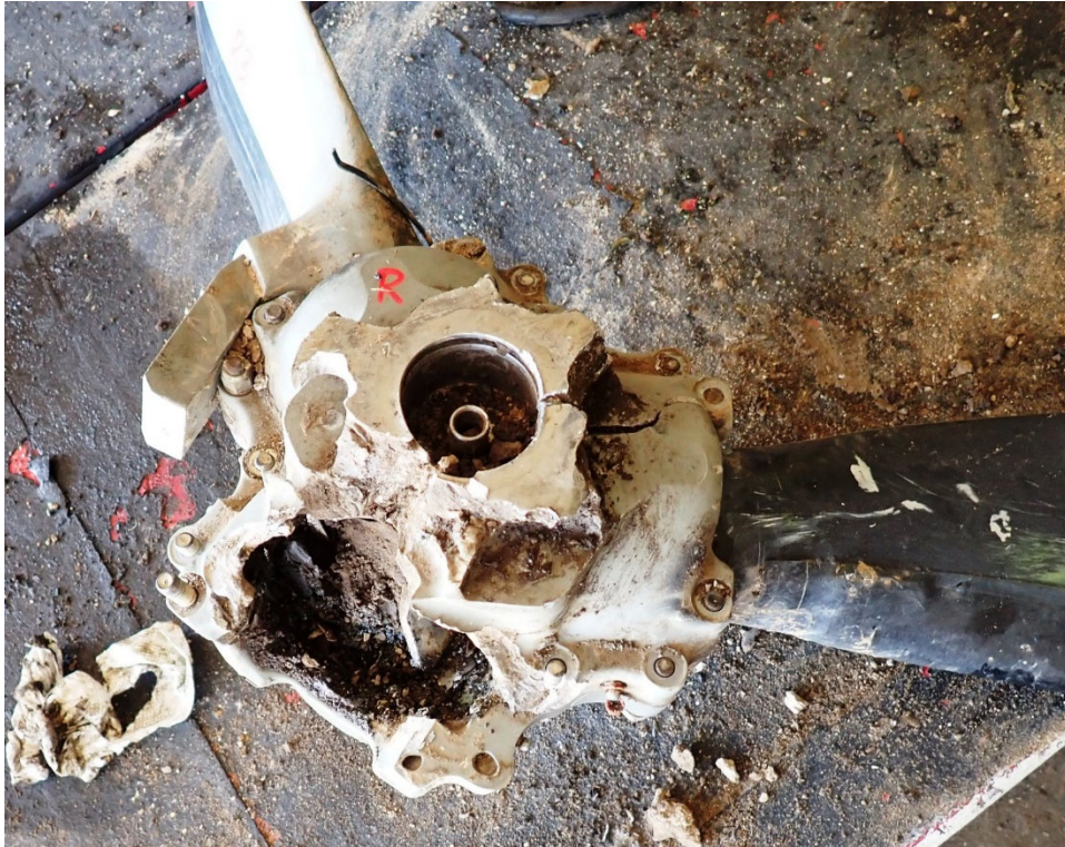
Photo #32 - R1 blade retention arm fractured
