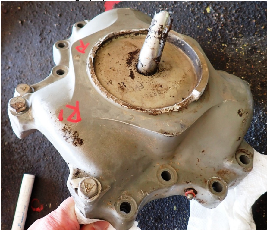
Photo #33 - Right propeller forward hub half – external view
