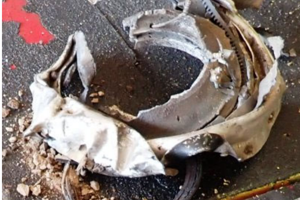
Photo #27 - Propeller spinner assembly remnants
