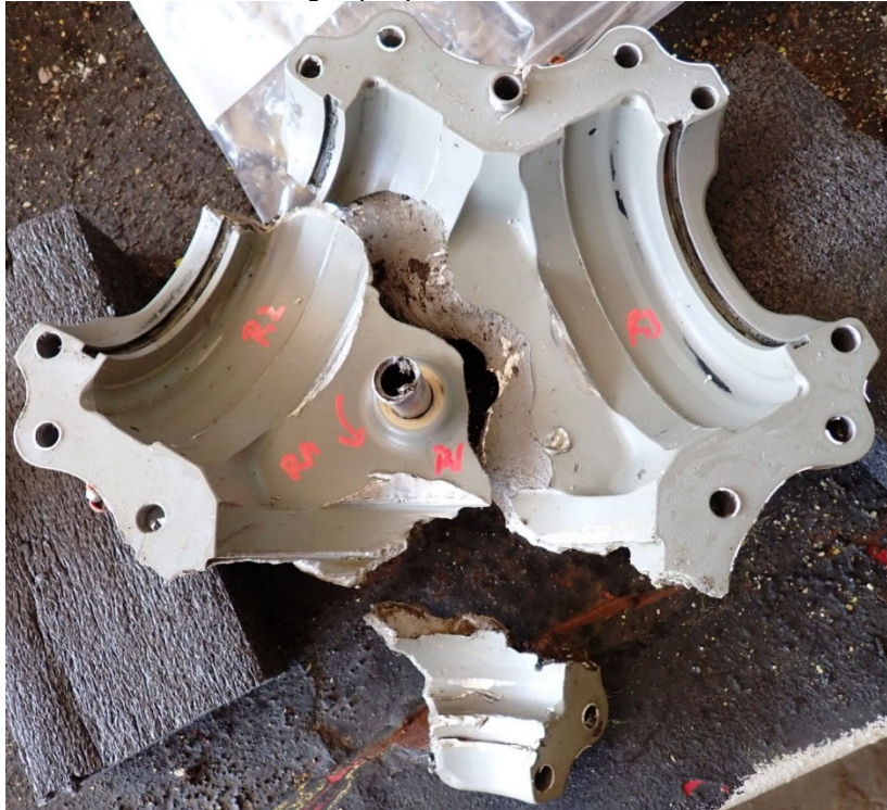
Photo #35 - Right propeller aft hub – internal view
