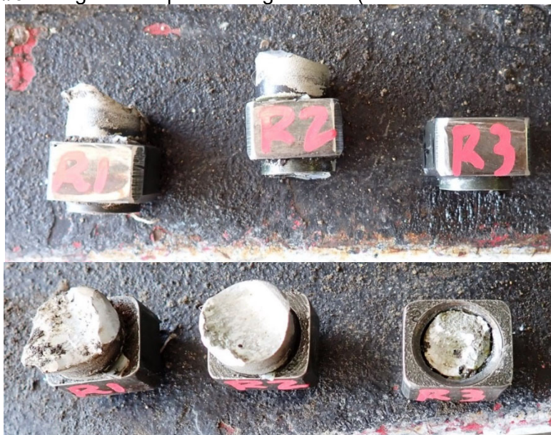
Photo #37 - Right blade pitch change blocks (R1 and R2 knobs fractured)
