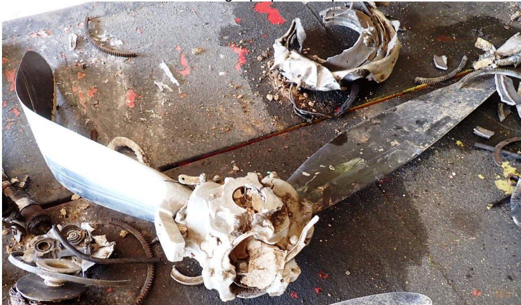
Photo #26 - Right propeller as-presented
