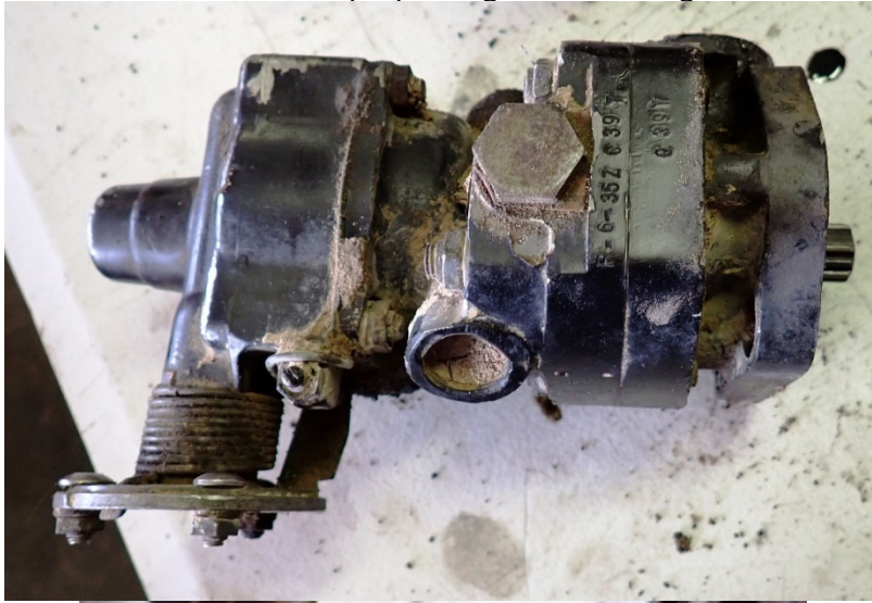
Photo #24 - Left propeller governor and gasket
