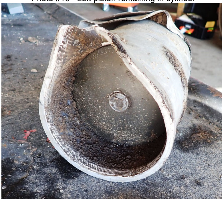
Photo #10 - Left piston remaining in cylinder
