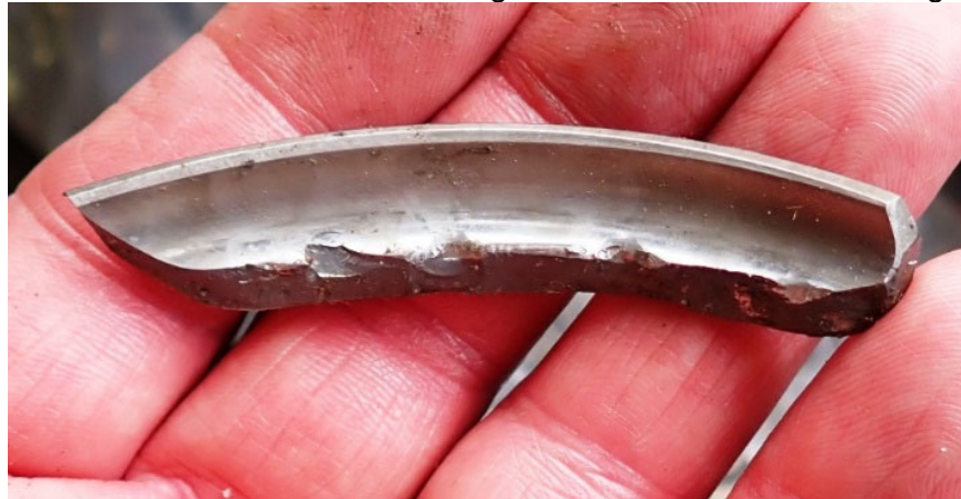
Photo #19 - Left blade retention bearing race fracture with ball bearing marks
