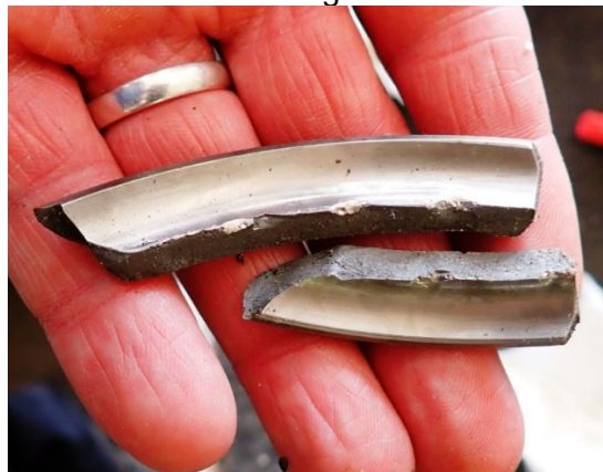
Photo #38 - Right blade retention bearing race fracture with ball bearing marks
