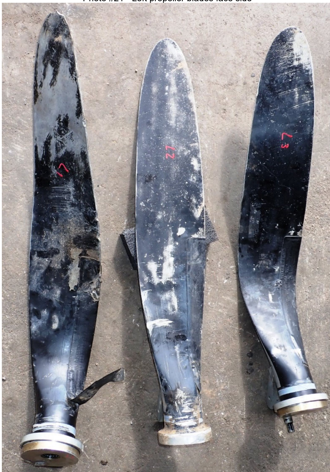
Photo #21 - Left propeller blades face side
