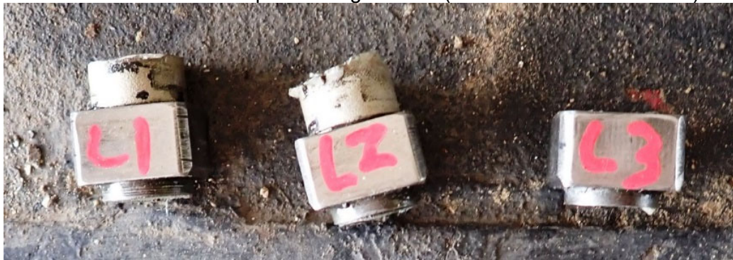
Photo #18 - Left blade pitch change blocks (L1 and L2 knobs fractured)
