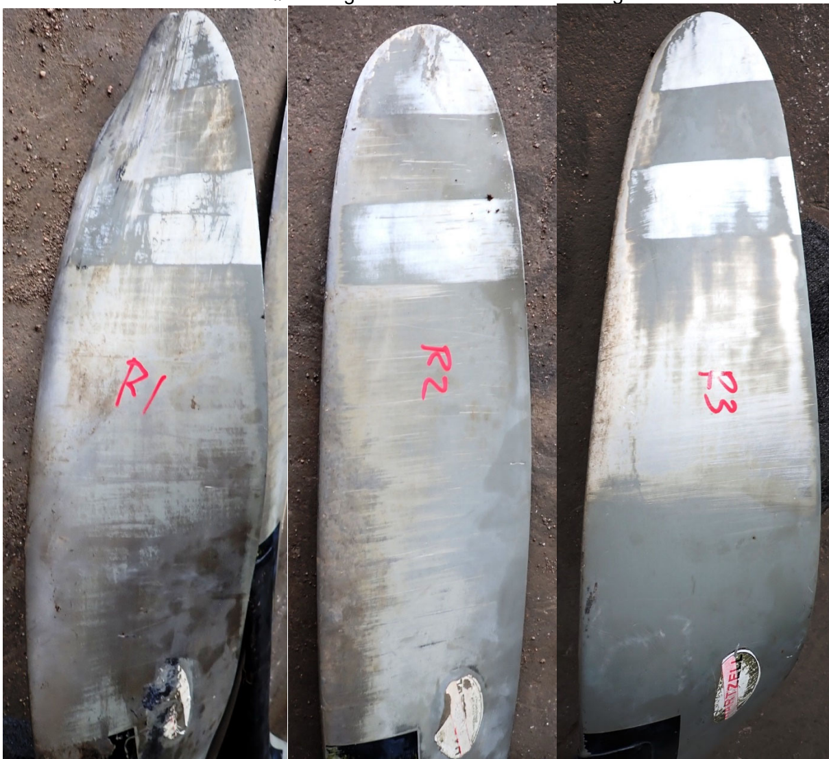
Photo #41 - Right blades camber-side scoring
