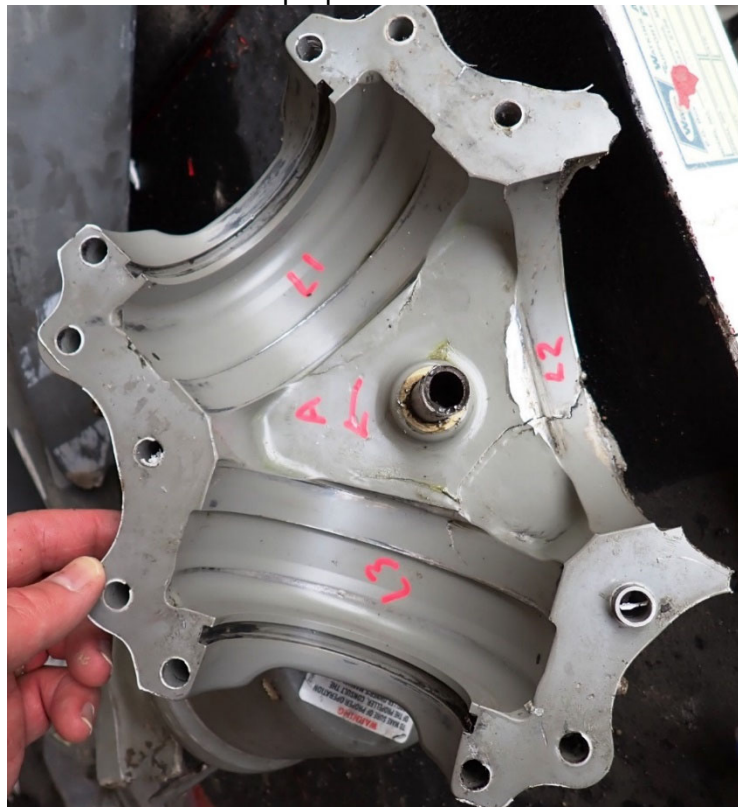
Photo #16 - Left propeller aft hub – internal view
