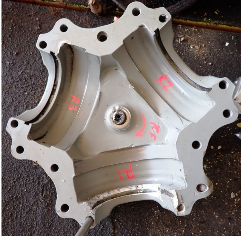
Photo #34 - Right propeller forward hub half – internal view
