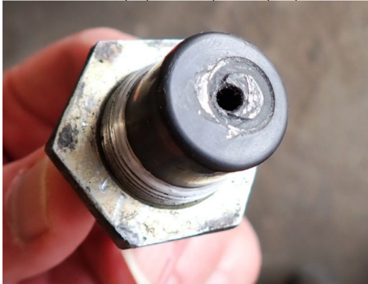
Photo #11 - Left propeller low pitch stop impact mark
