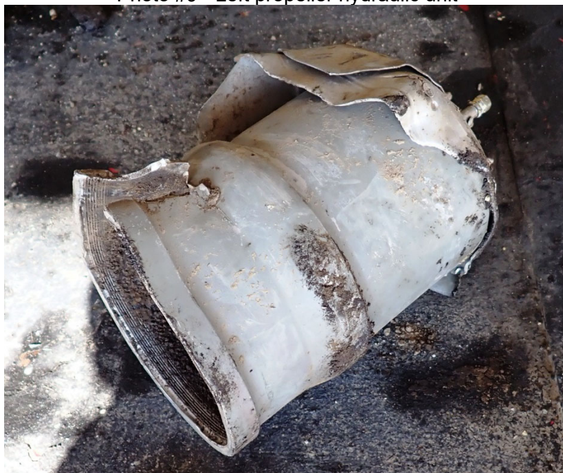
Photo #9 - Left propeller hydraulic unit
