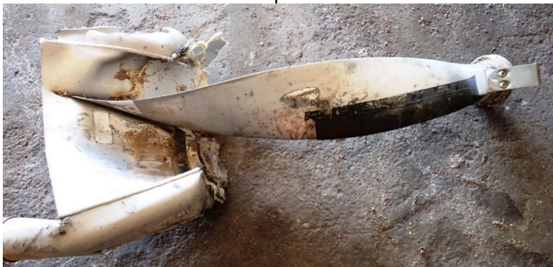
Photo #28 - Blade R1 impaled the turbo intercooler
