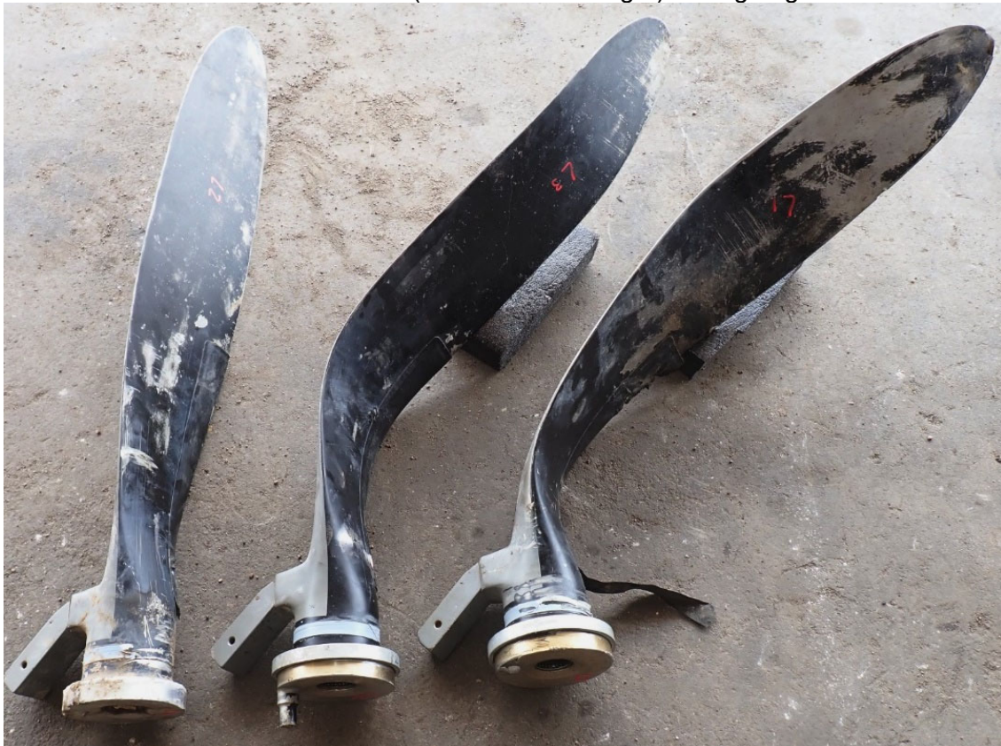
Photo #23 - Left blades (L2-L3-L1 left-to-right) trailing edge view
