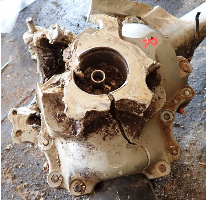
Photo #30 - Right propeller hub mounting flange
