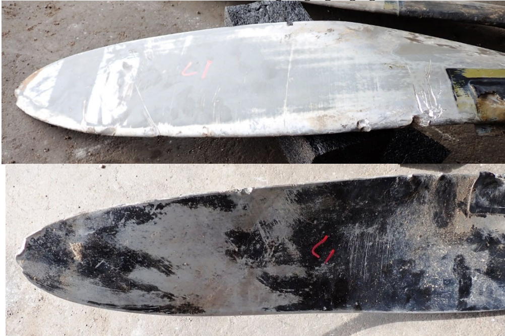
Photo #22 - L1 leading edge gouging
