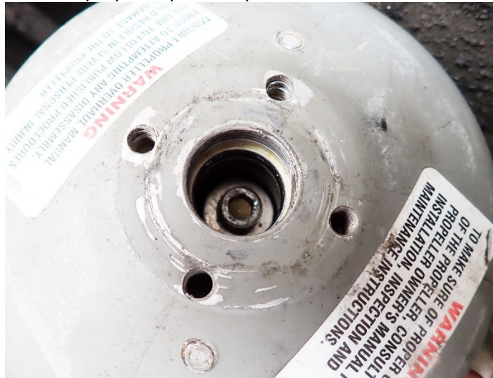
Photo #12 - Left propeller pitch stop stack intact and near the start lock
