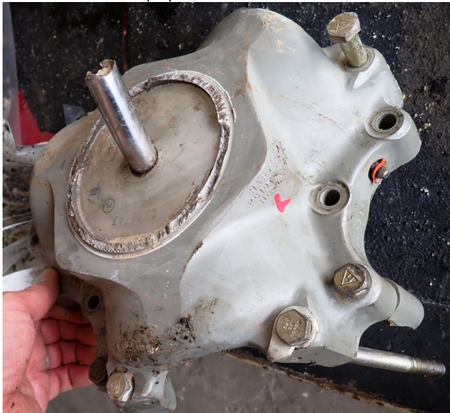
Photo #14 - Left propeller forward hub half – external view
