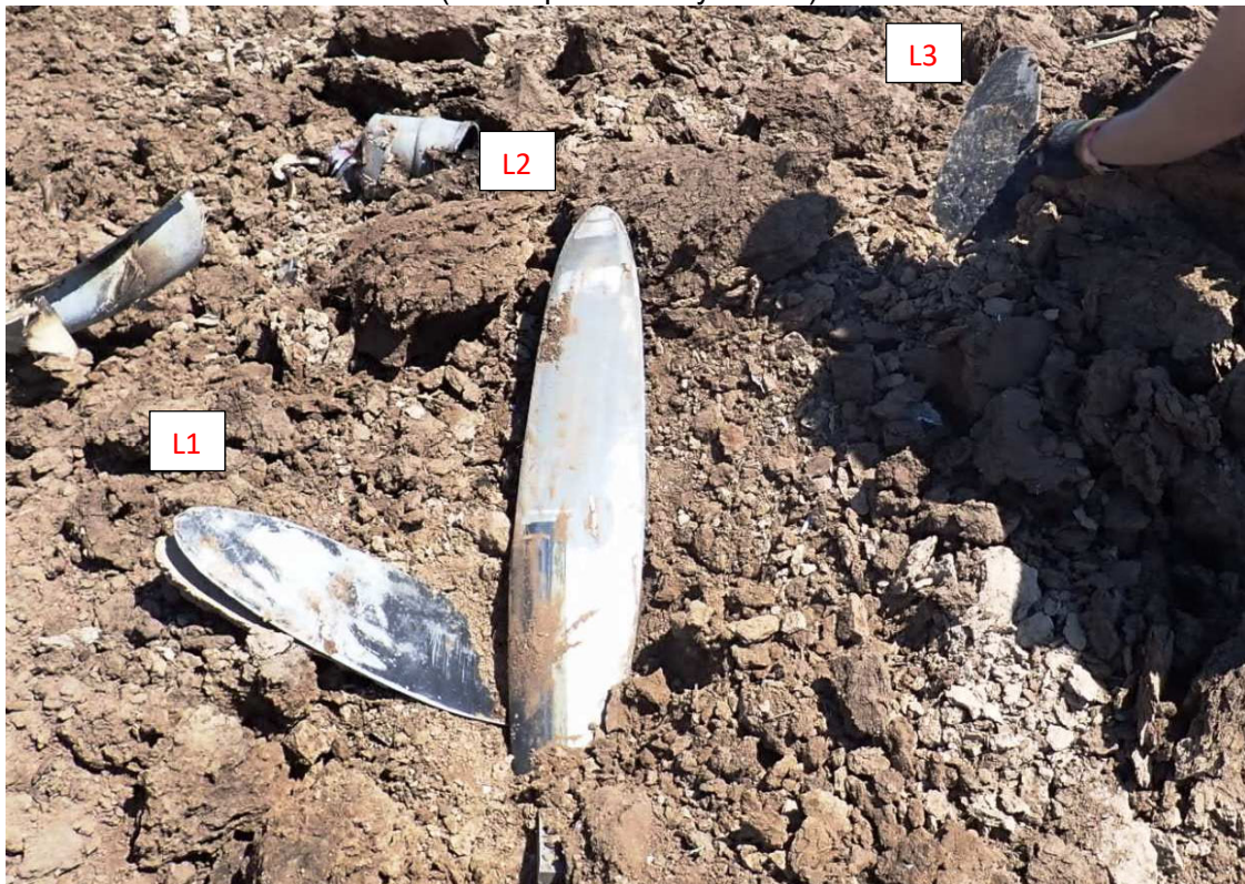
Photo #4 - Left propeller in-situ (Photo provided by NTSB)
