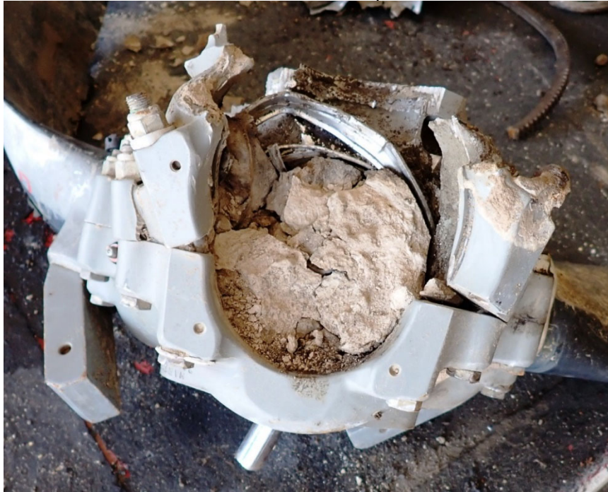
Photo #13 - L2 blade retention pocket fractured
