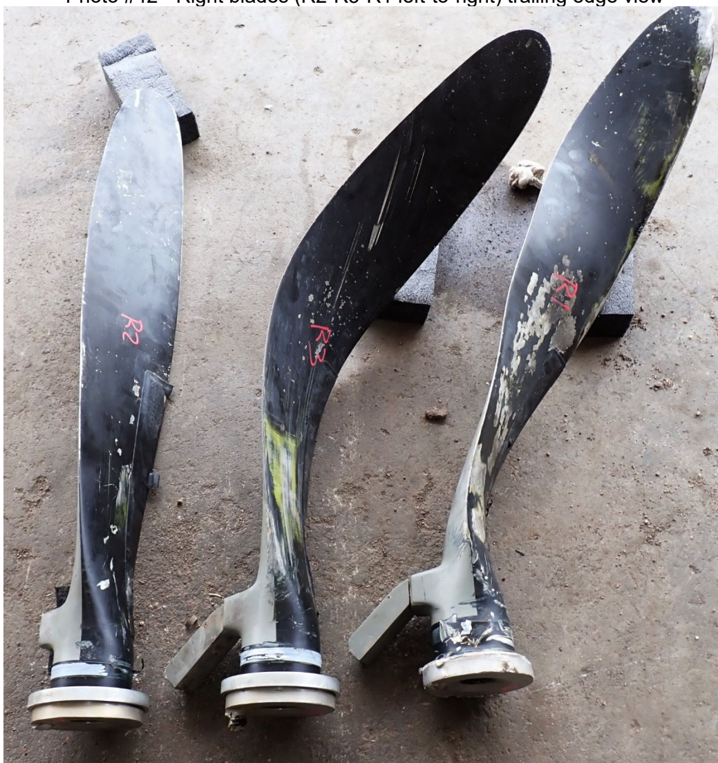
Photo #42 - Right blades (R2-R3-R1 left-to-right) trailing edge view
