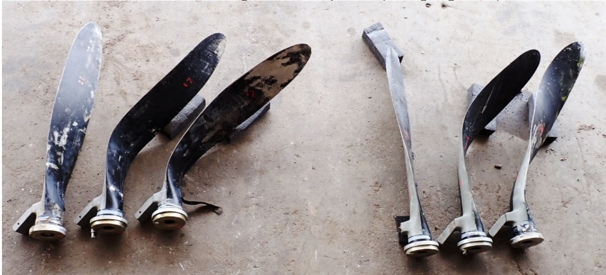
Photo #3 - Left vs. Right blade comparison (trailing edge view)
