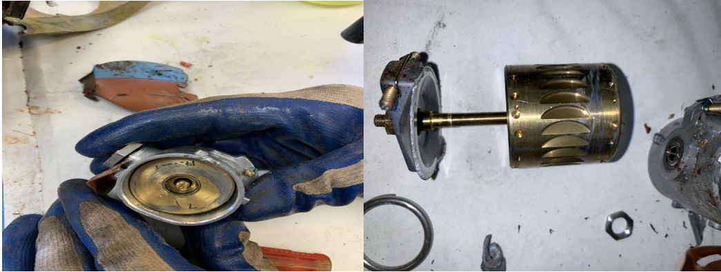
Figure 2 - Attitude Indicator Housing and Gyro
