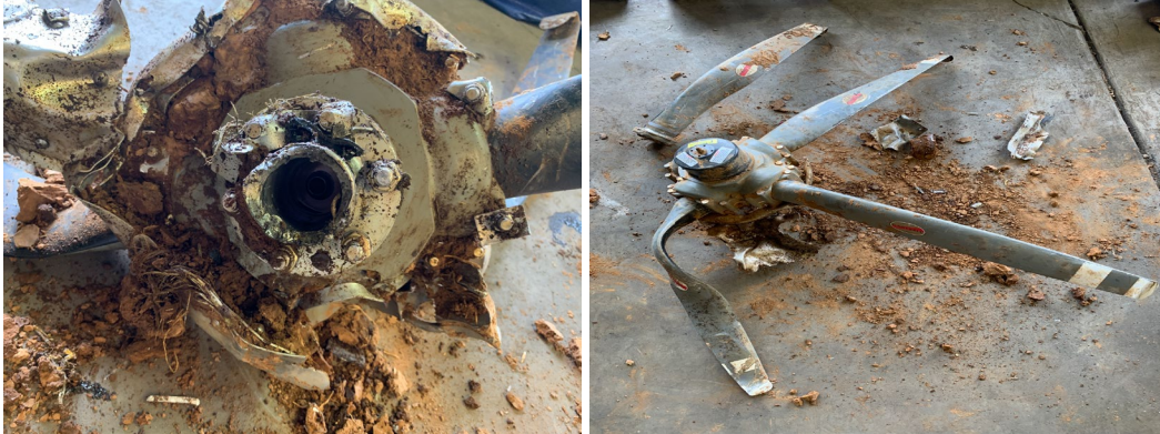
Figure 4 - Propeller Flange and Blades
