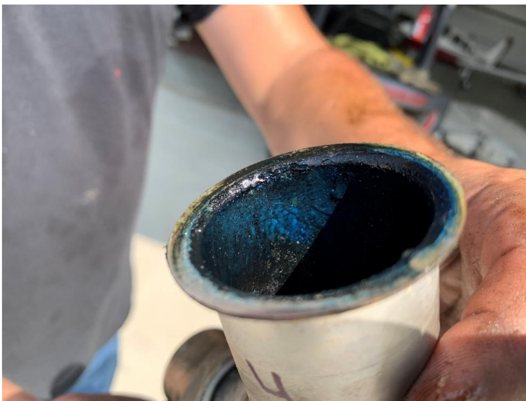
Figure 6. Intake tube with fuel staining.
