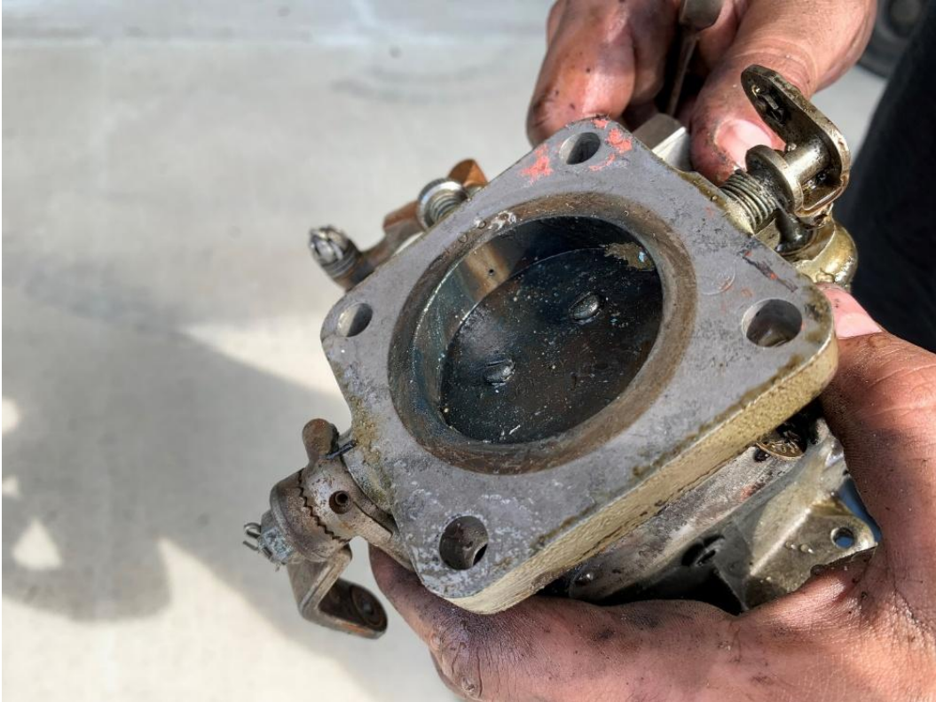
Figure 7. Fuel staining on throttle plate and carburetor throat.
