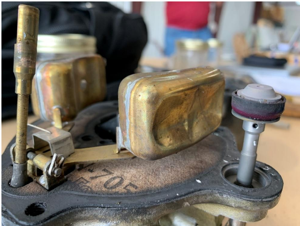
Figure 8. Hydraulic deformation to carburetor float.
