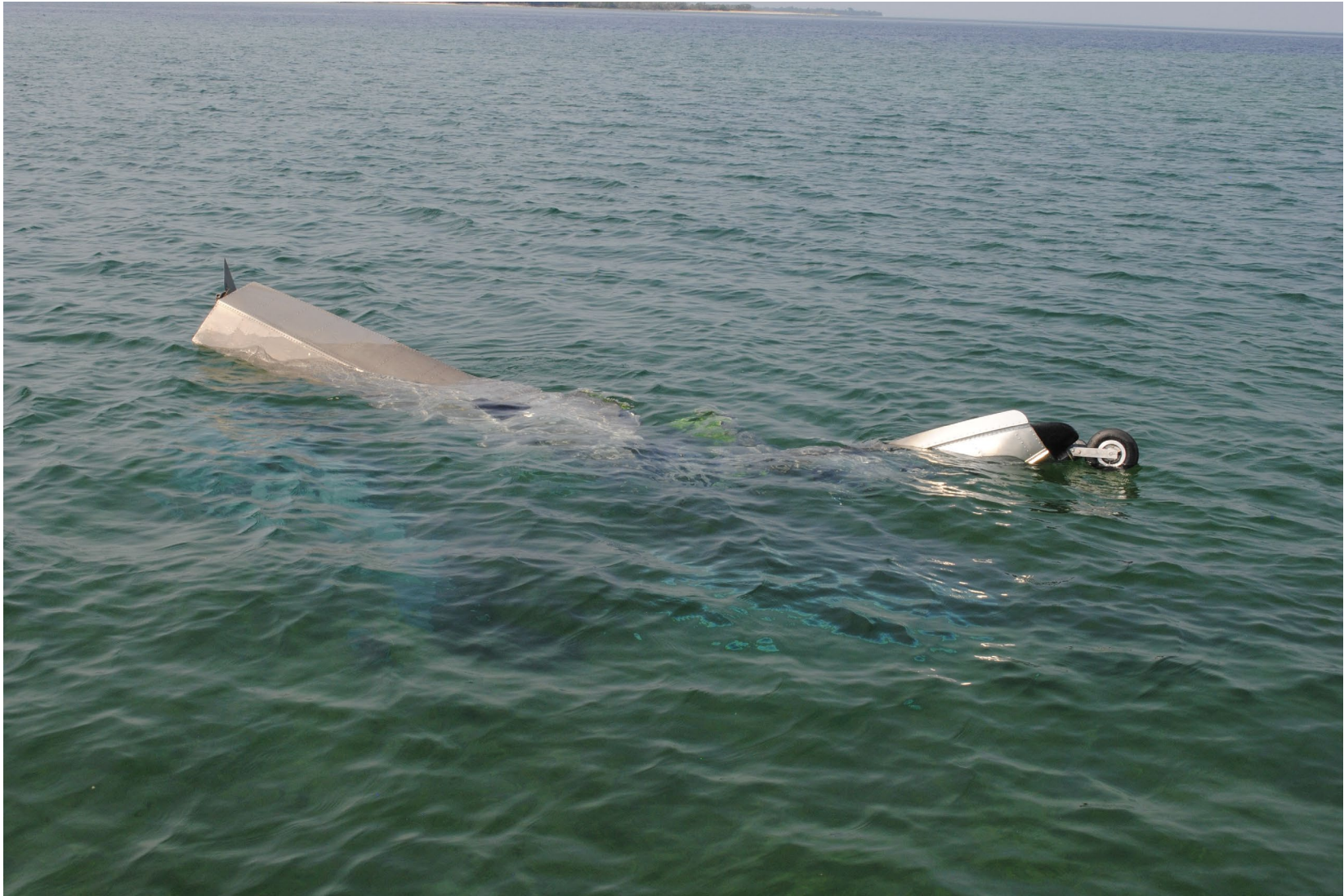
Photograph 2 - Airplane floats separated from airplane. (Courtesy of LEO)
