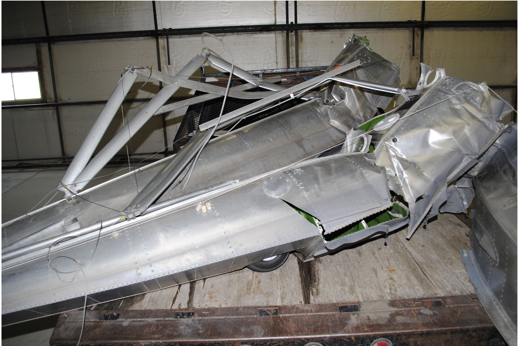
Photograph 5 - Floats exhibiting significant crush damage (Courtesy of LEO)
