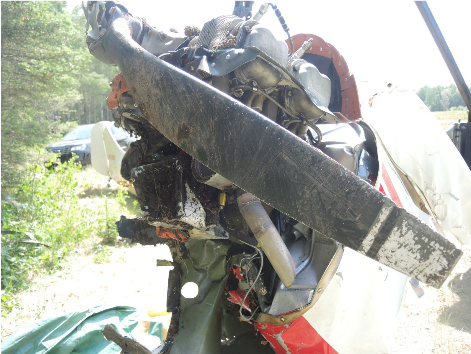
Photograph 9 - Propeller Damage (Courtesy of NTSB)
