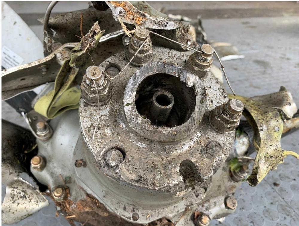
Figure 11. Engine propeller flange and portion of crankshaft
