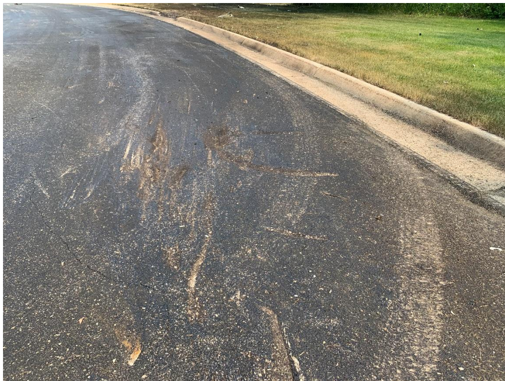
Figure 2. Airplane impact with road and propeller slash marks
