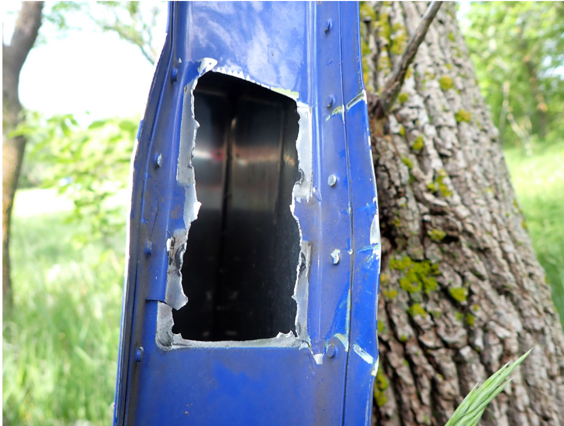
Photograph 5 - Vertical stabilizer where rudder hinge was torn away
