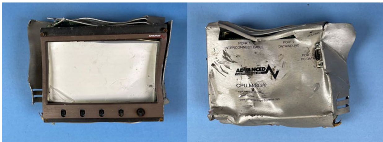
Figure 1. Front view (left) and back view (right) of Advanced Flight Systems AF-2500, as received by the NTSB Vehicle Recorder Laboratory.
