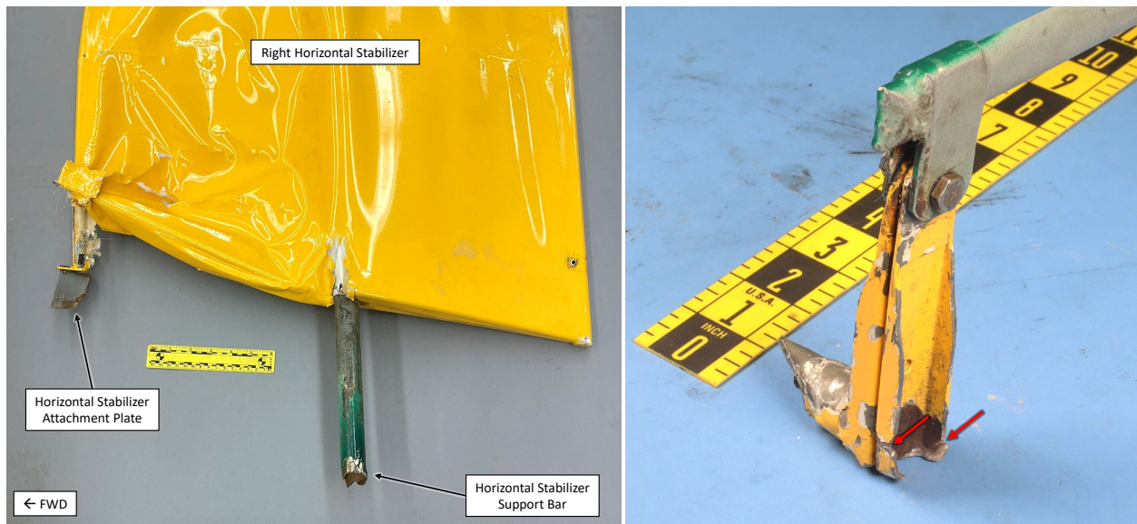
Figure 23. Photographs of the separated right horizontal stabilizer (left) and fractured right elevator horn attachment location (right).
