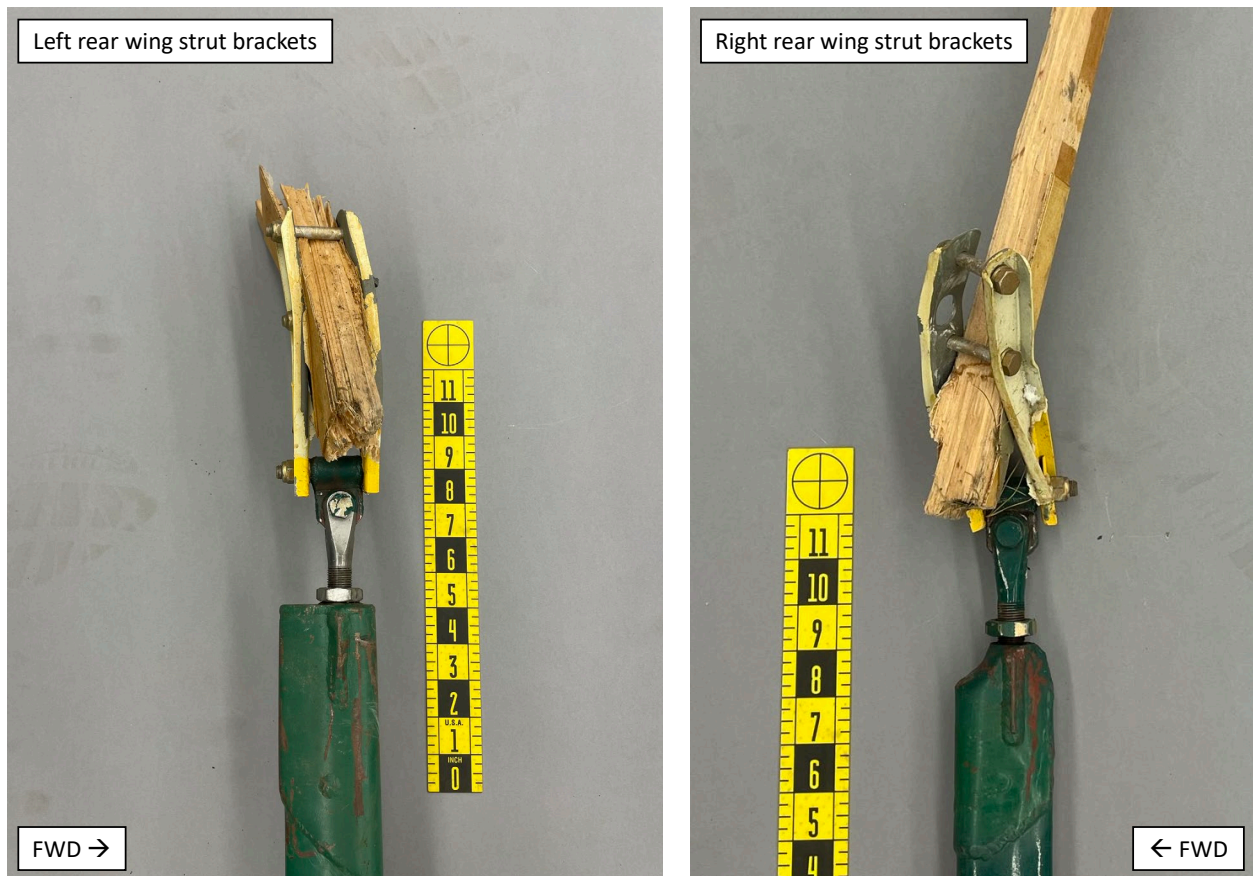
Figure 21. Photographs of the rear strut brackets as viewed looking down showing torsional bending deformation and pieces of retained rear spar.
