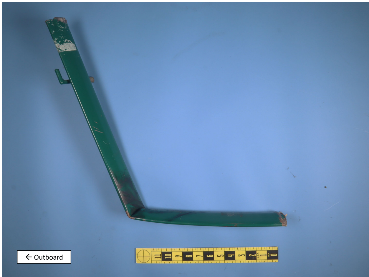
Figure 13. Photograph of the outboard end of the fractured left front wing strut. A black material transfer mark was observed on the upper surface spanning the region which was buckled upward.
