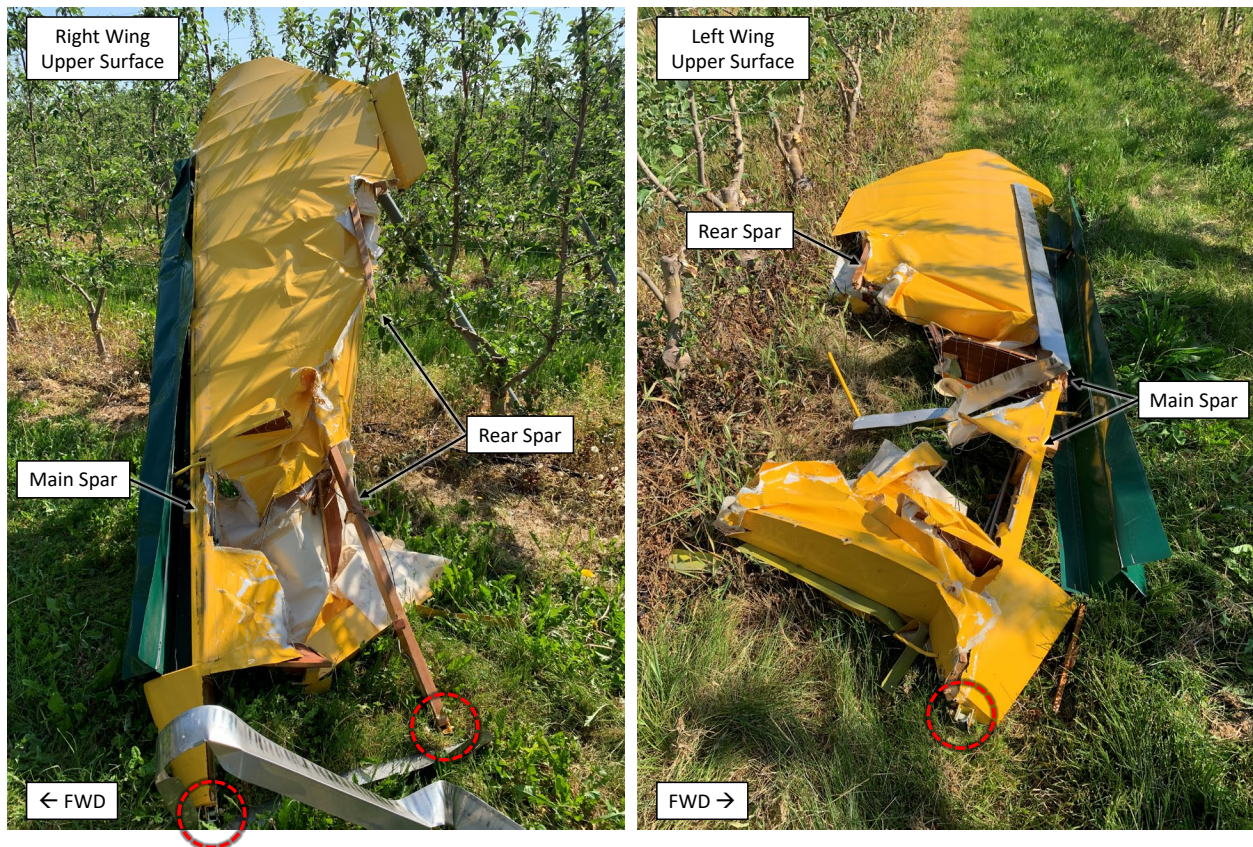
Figure 2. On-scene photographs showing right wing (left image) and left wing (right image). Retained wing attachment brackets are circled in red.
