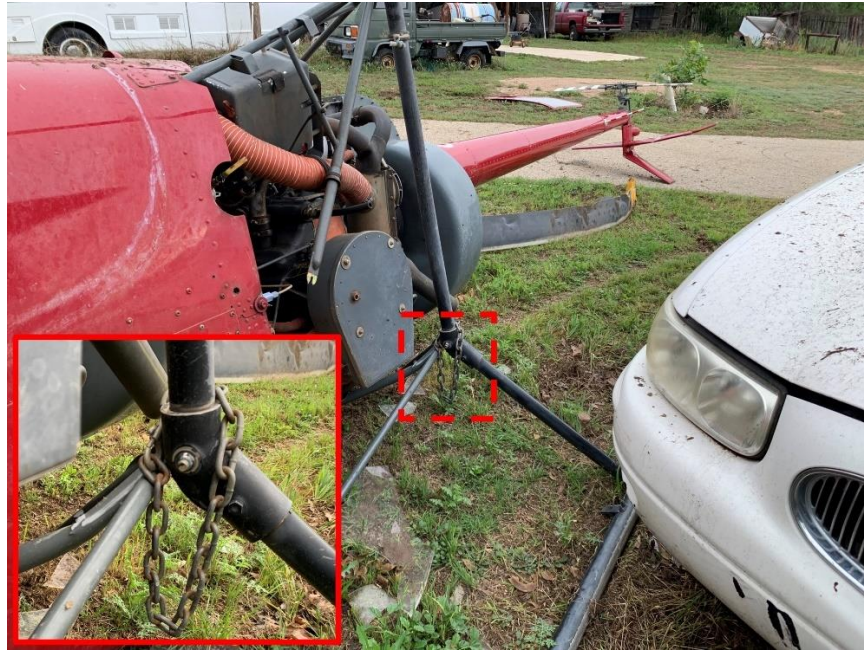
Figure 7. Chain loop around the landing gear skid aft cross tube.
