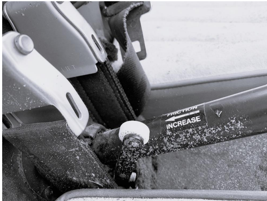
Figure 6. Collective friction in off position.
