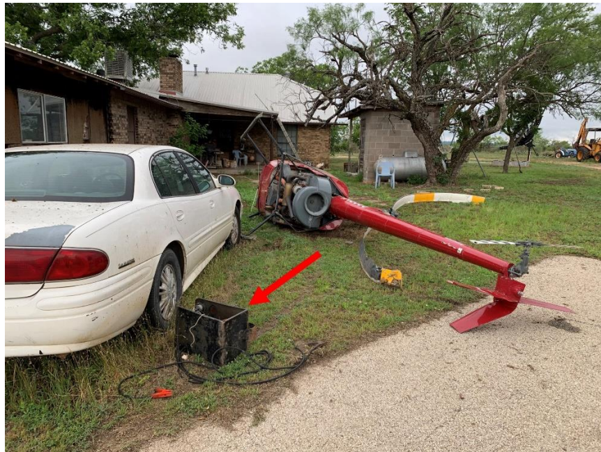
Figure 4. Main wreckage, sedan, and battery charger with jumper cables (red arrow).
