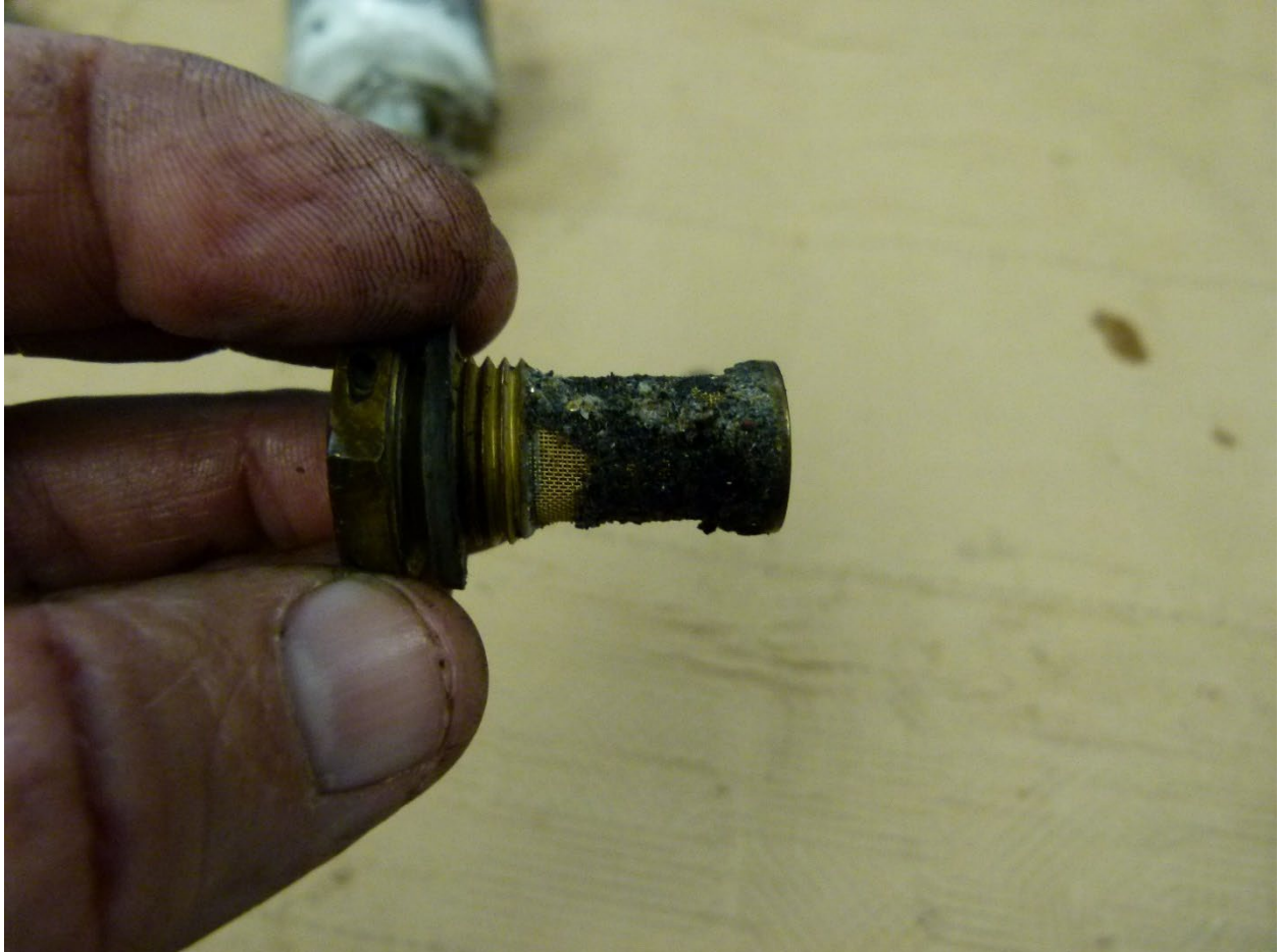
Photograph 1. Fuel plug and screen assembly from right engine (Photo from NTSB)
