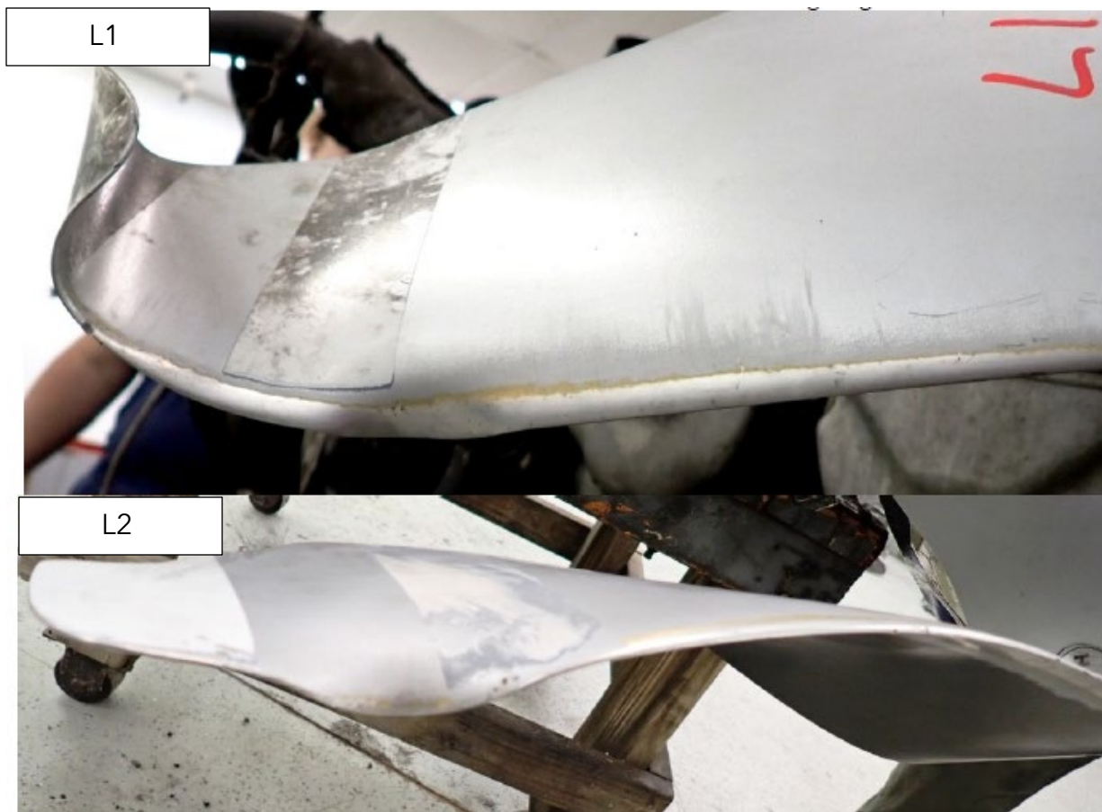
Photo 6. Tree strike bends in L1 and L2 leading edges
