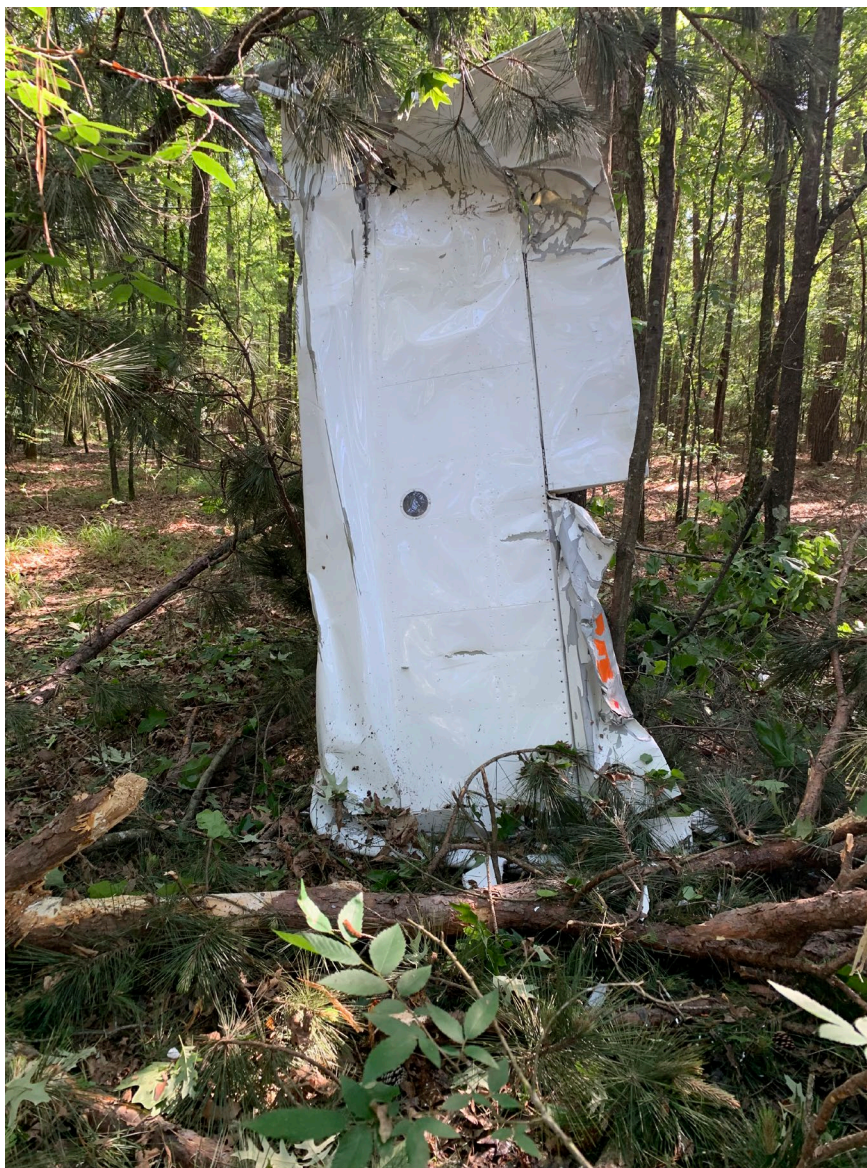
Photograph 3 - Separated Left Wing after Recovery (Courtesy of NTSB)
