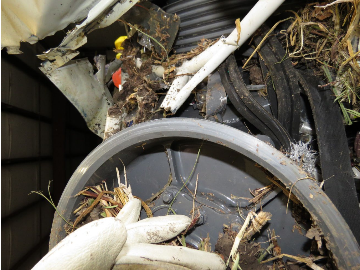
Figure 5. Rotational scoring on the forward surface of the upper sheave (Source: Robinson Helicopter).
