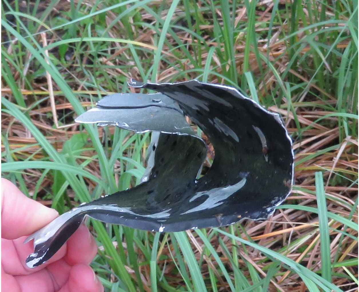
Figure 15. Separated metal from above camera gimbal mount consistent with main rotor blade impact (Source: Robinson Helicopter).
