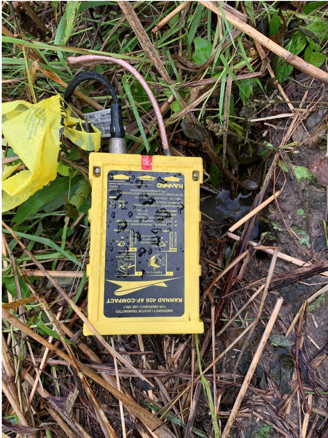
Figure 17. ELT located in the debris field with antenna wire severed.
