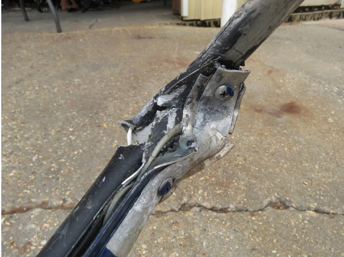
Figure 14. Top of windshield bow consistent with main rotor blade impact (Source: Robinson Helicopter).
