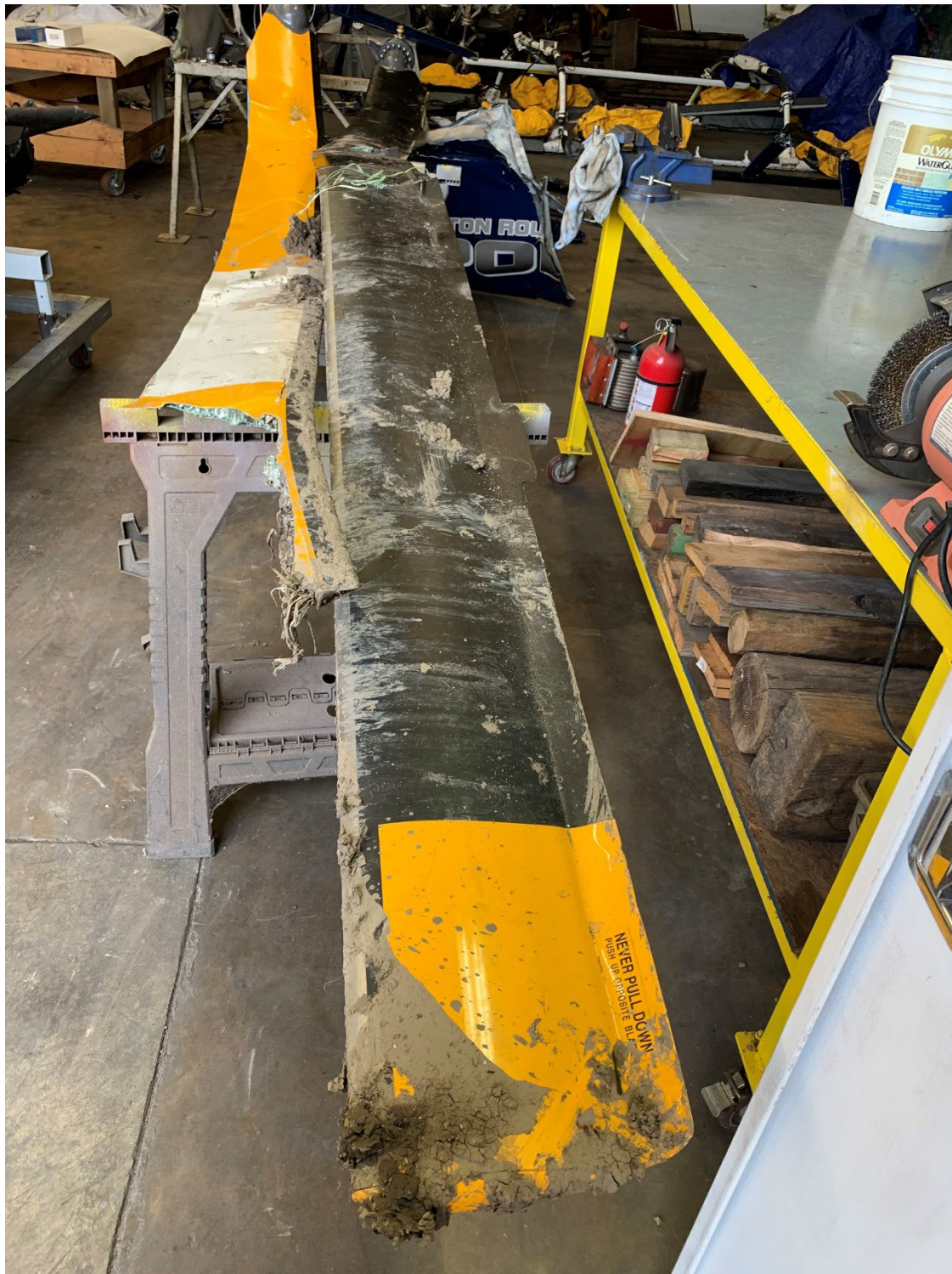
Figure 11. Main rotor blades and damage.
