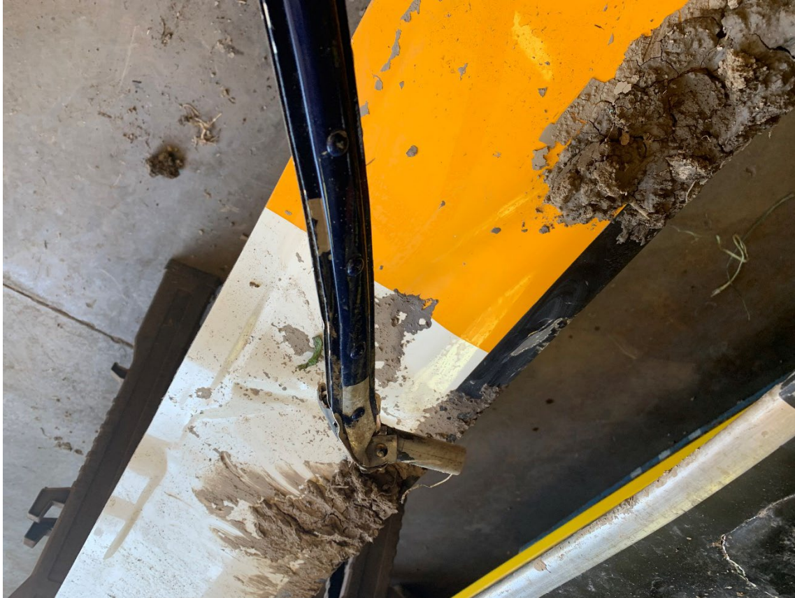
Figure 16. Windshield bow and corresponding main rotor blade impact.
