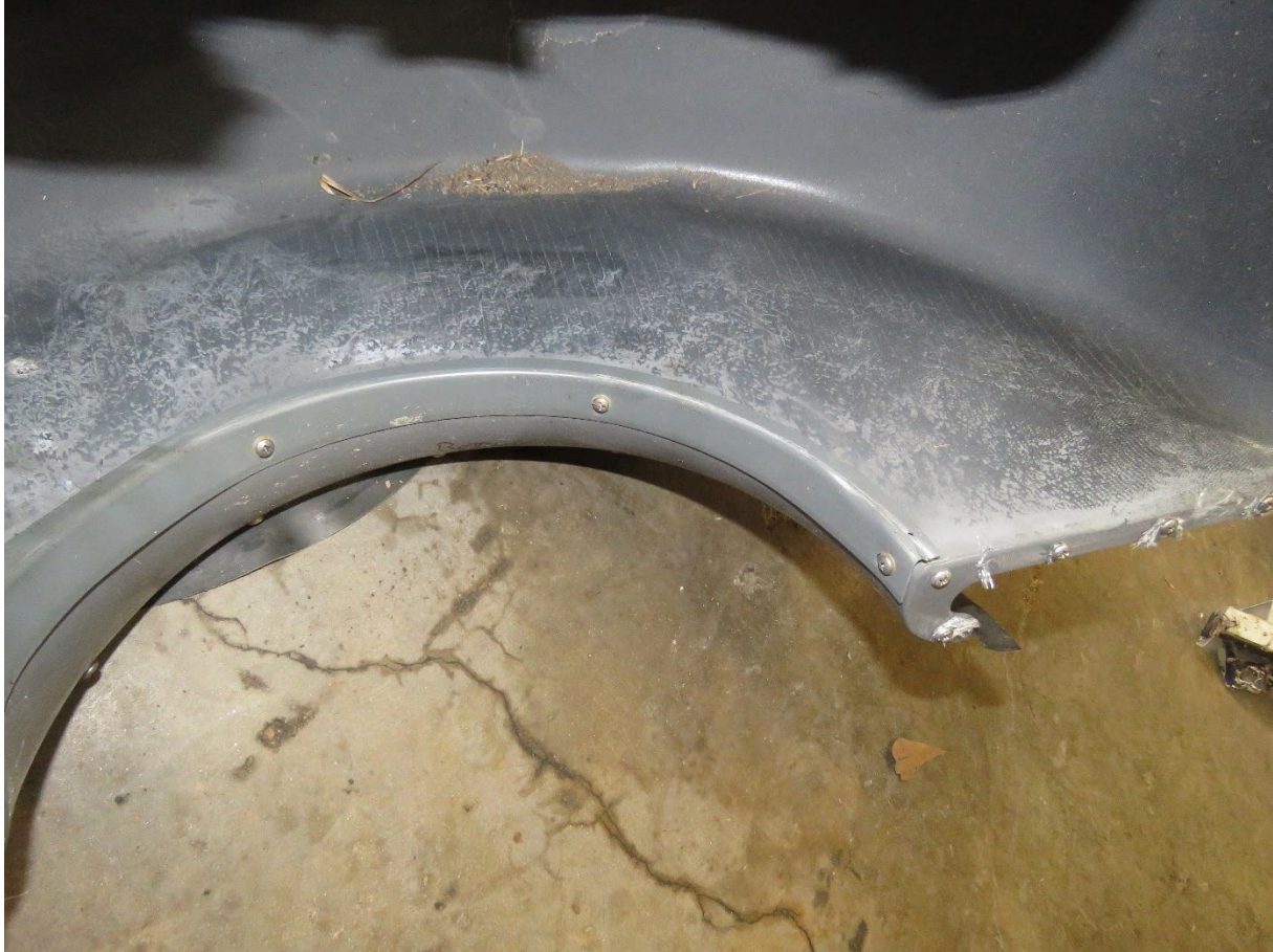
Figure 6. Rotational scoring on the lower half of the fan scroll (Source: Robinson Helicopter).
