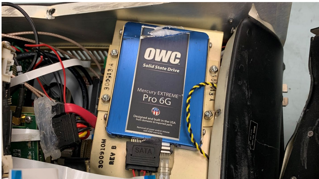
Figure 3. AeroComputers UC-5300 internal SSD, as received.
