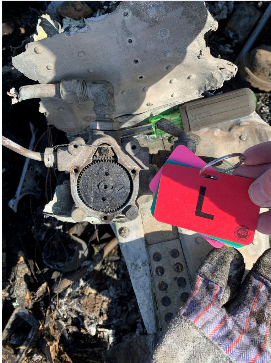
Photograph 3 - Left Fuel Selector Assembly (By NTSB ICC)
