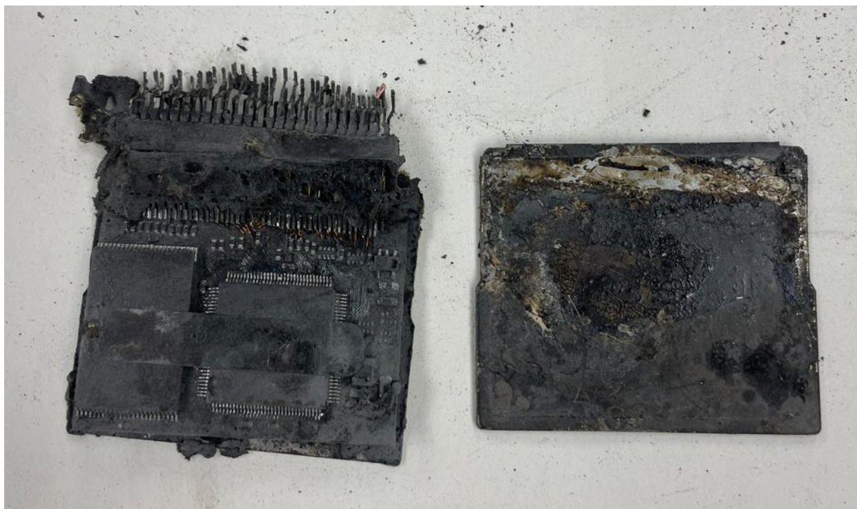
Figure 4. Internal of the Avidyne IFD 440 compact flash card.
