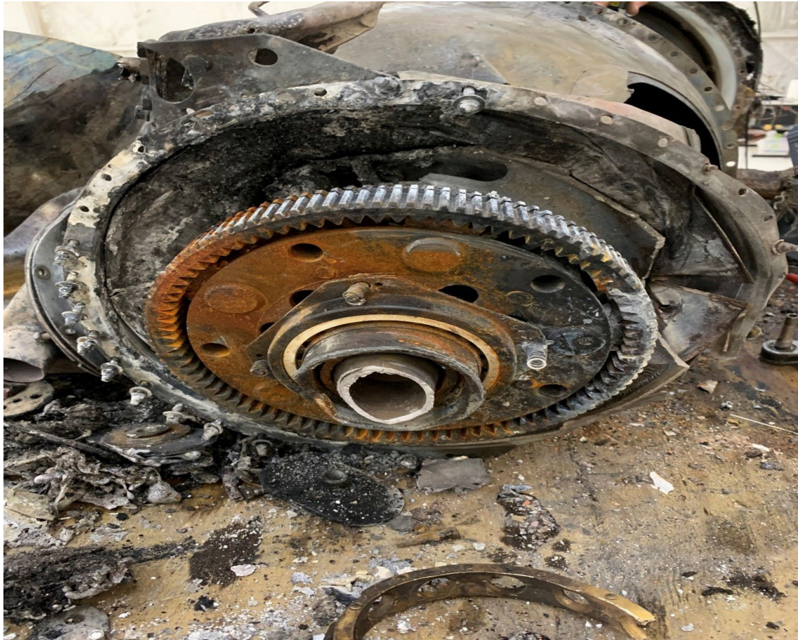
Photograph 5 - Right Engine Sun Gear and Fractured Propeller Shaft
