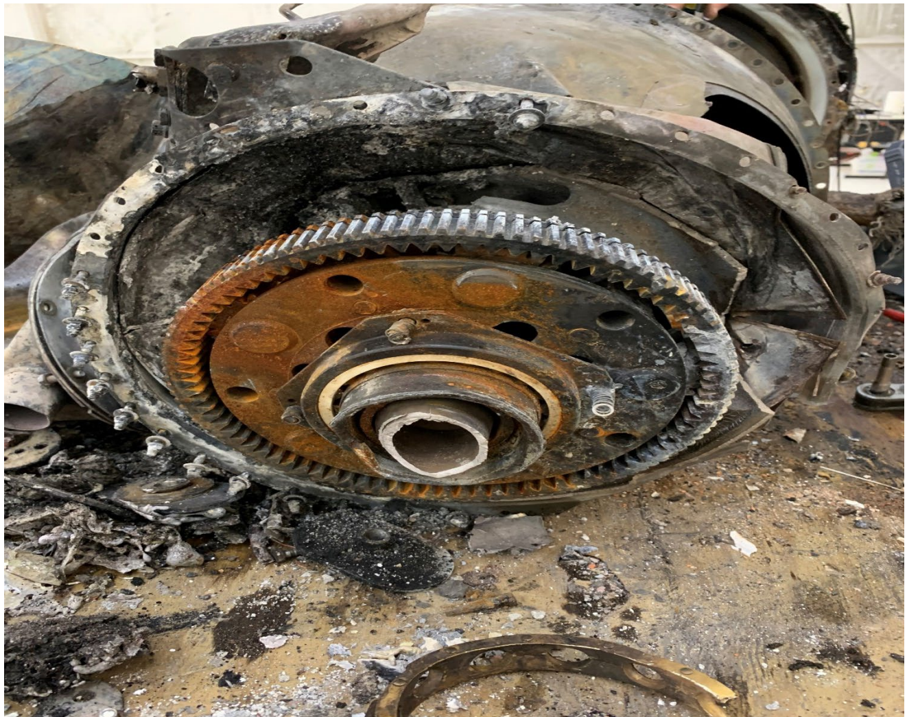
Right Engine Sun Gear Assembly and Fractured Propeller Shaft
