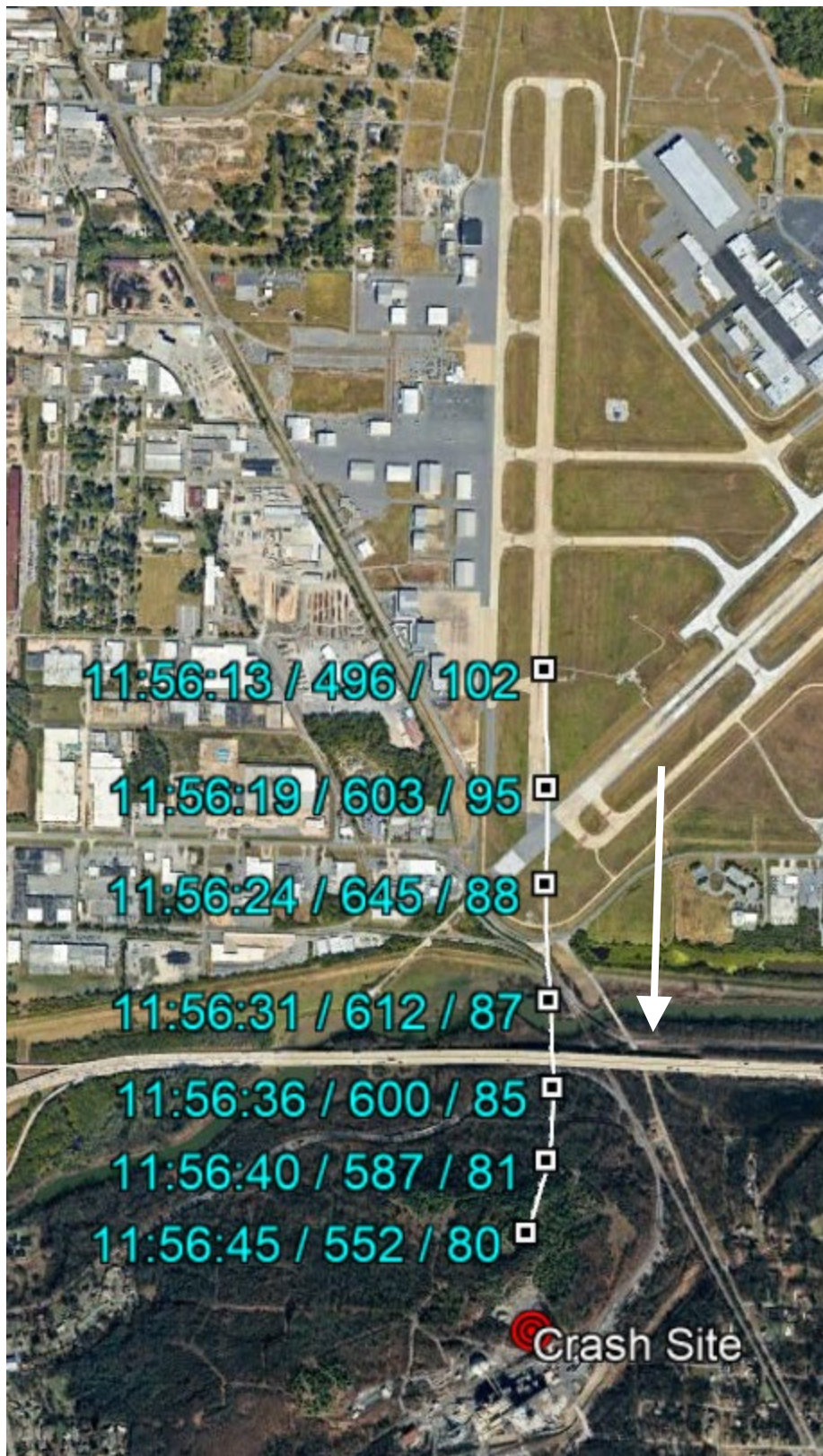
Figure 4. Overhead view of the accident flight path. Annotations indicate the time, altitude msl and groundspeed. North is at the top.
