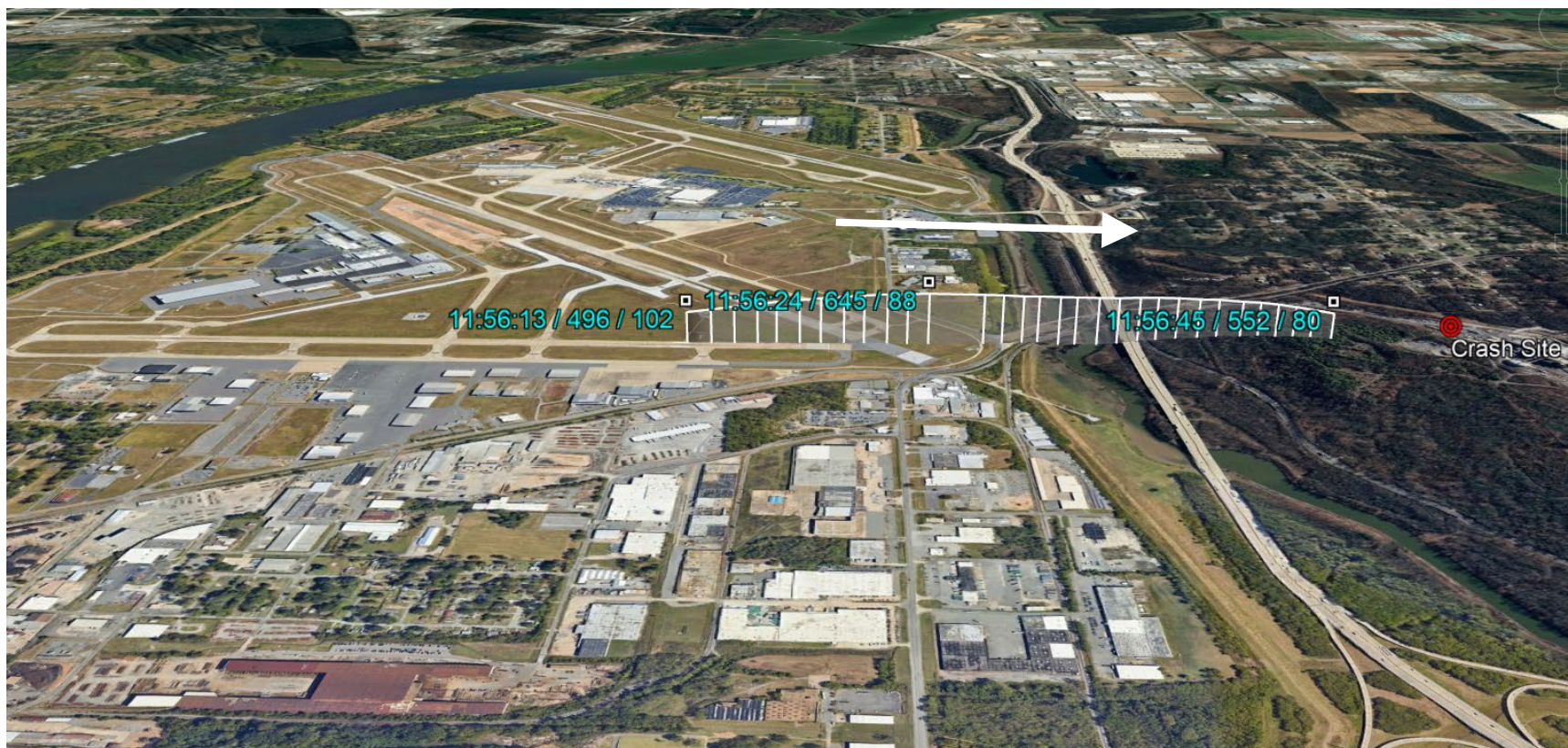
Figure 3. Profile view of the accident flight path. Annotations indicate the time, altitude msl and groundspeed. North is to the left.
