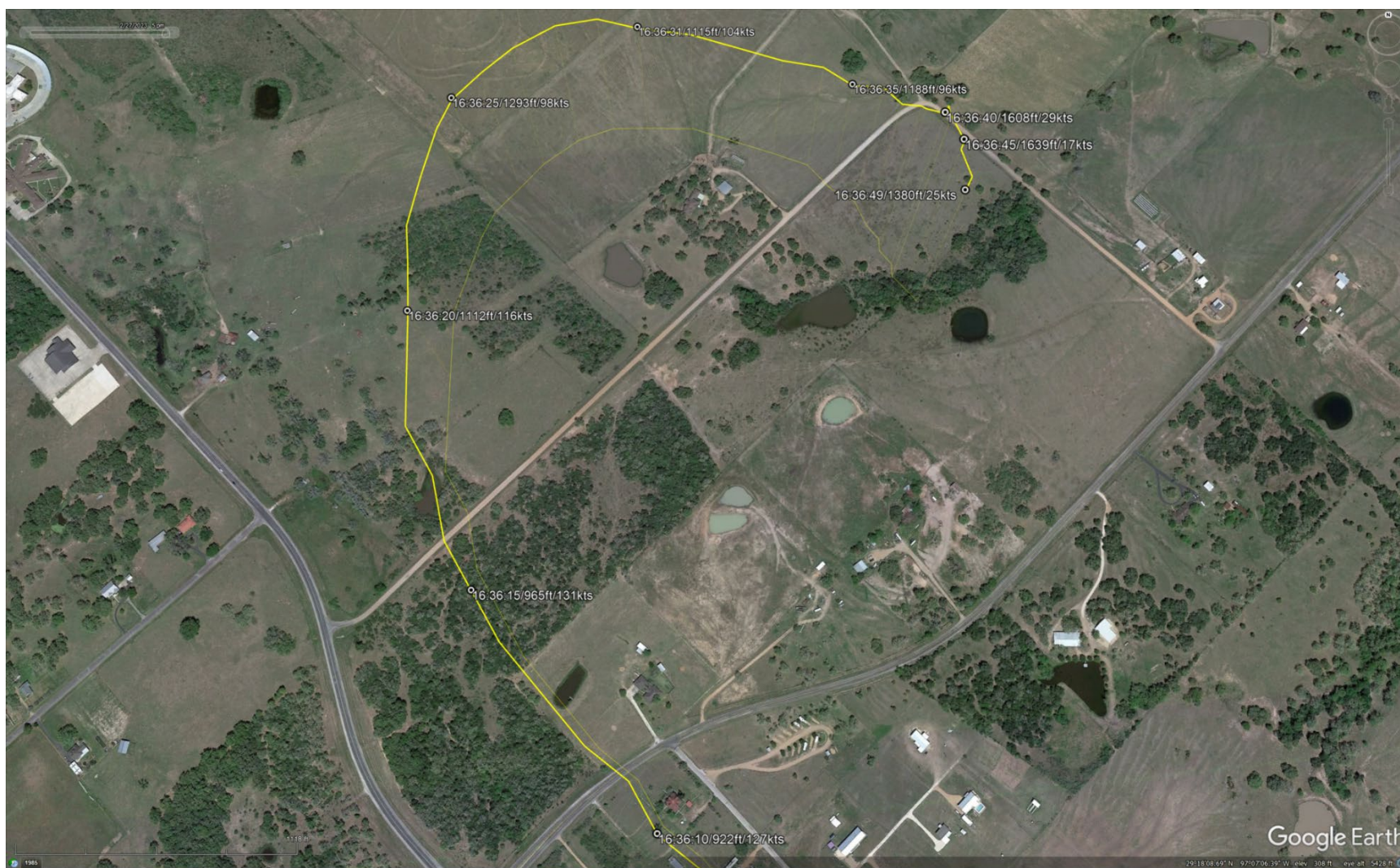
Figure 9. Google Earth overlay of final minute of the accident flight recorded on the Electronics International MVP-50T.
