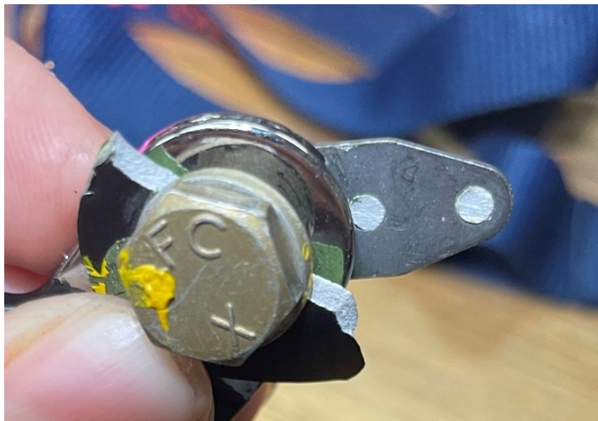
Figure 13. Close up view of the seat 6 outboard anchor with through bolt still secured.
