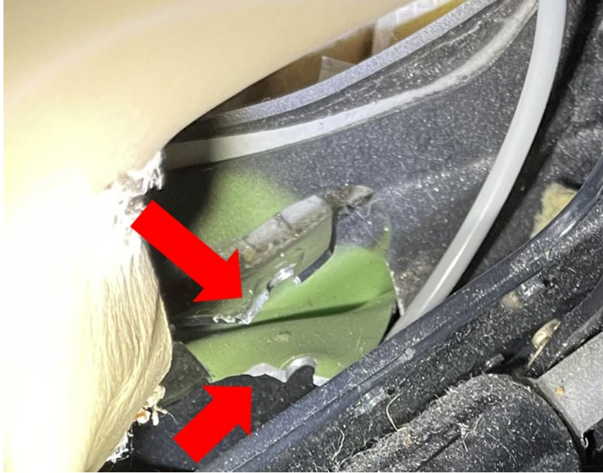
Figure 14. Seat 6 outboard anchor point airplane bracket, red arrows point to failed portion of the bracket.
