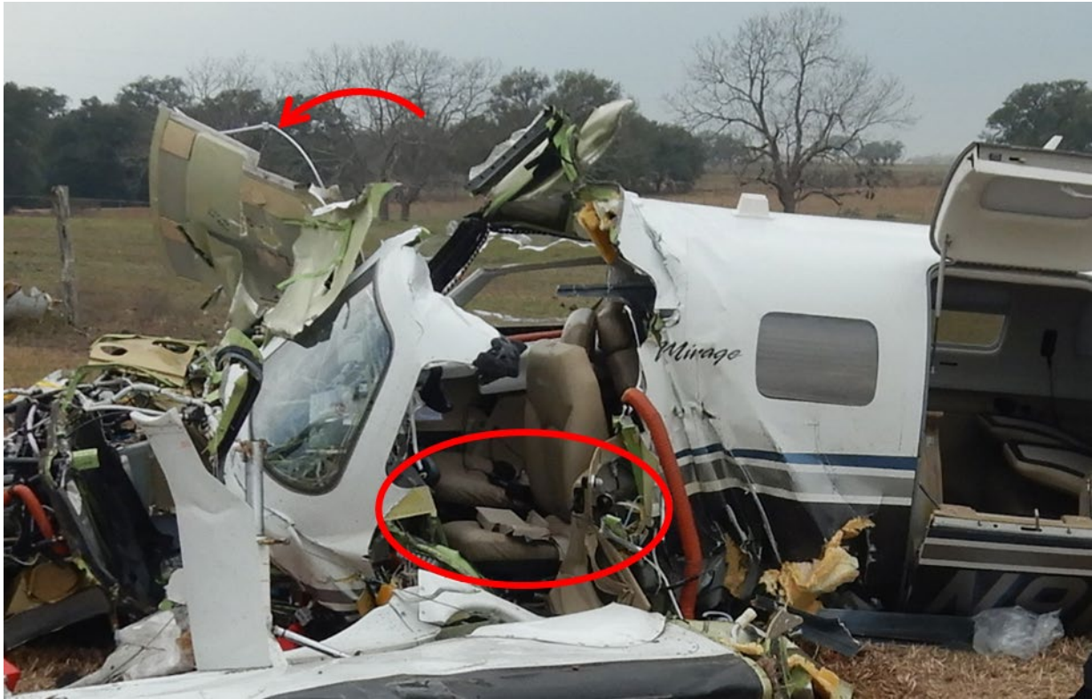
Figure 8. The cockpit area marked where emergency services moved structure to remove the occupants.
