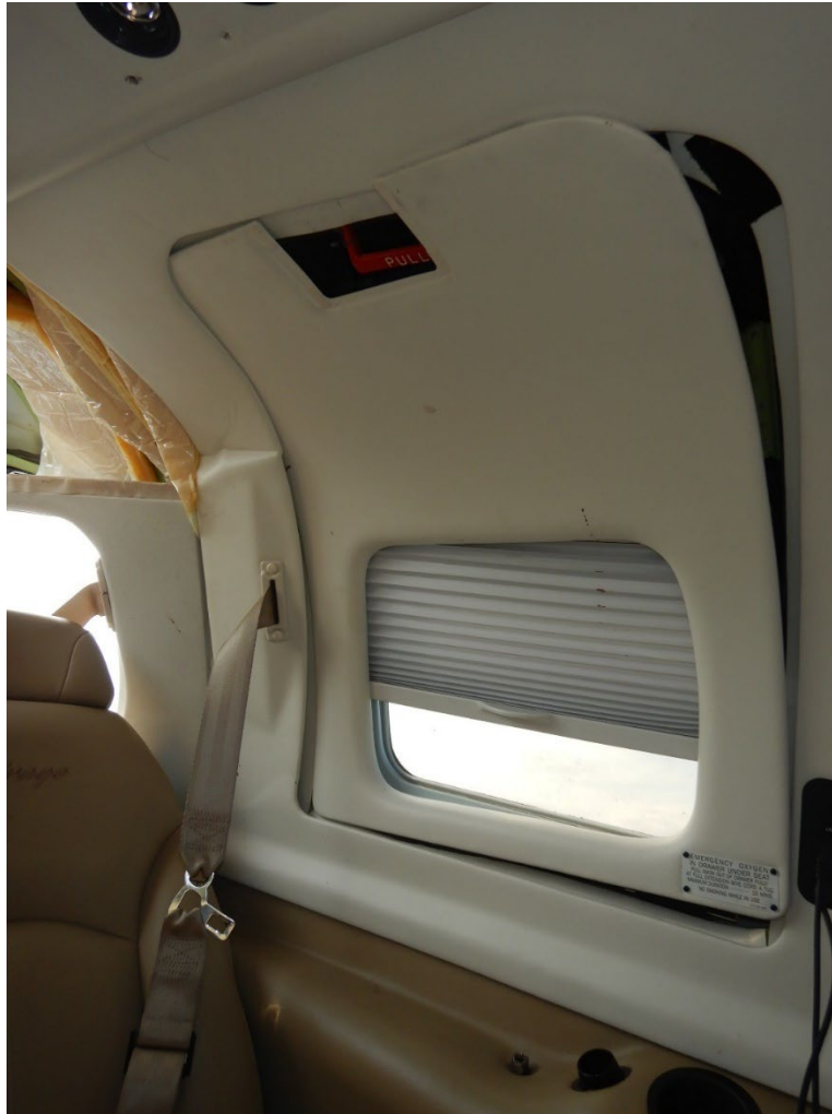
Figure 7. Emergency exit as found by investigators at the accident site. (Source: Piper Aircraft).
