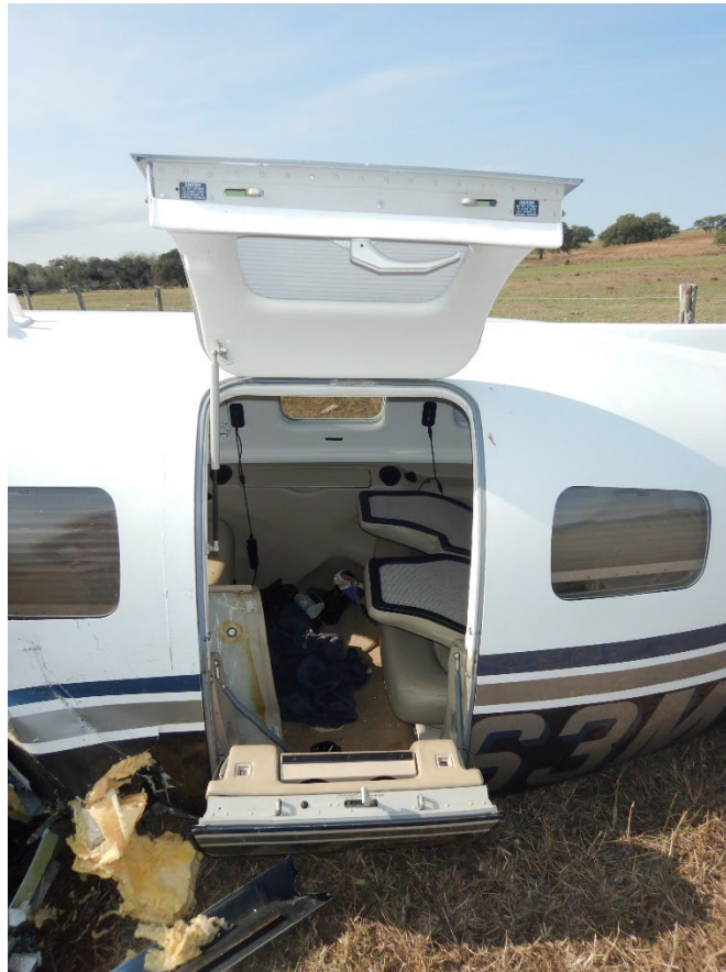
Figure 6. Main door as found by investigators at the accident site. (Source: Piper Aircraft)
