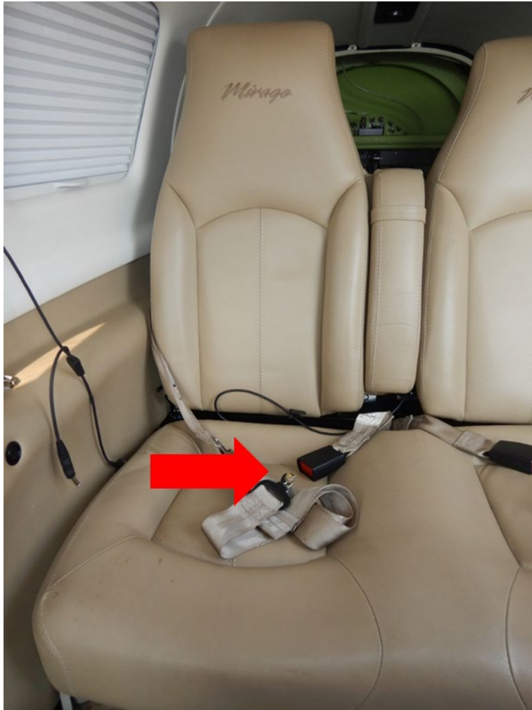
Figure 12. Outboard anchor failure at seat 6.
