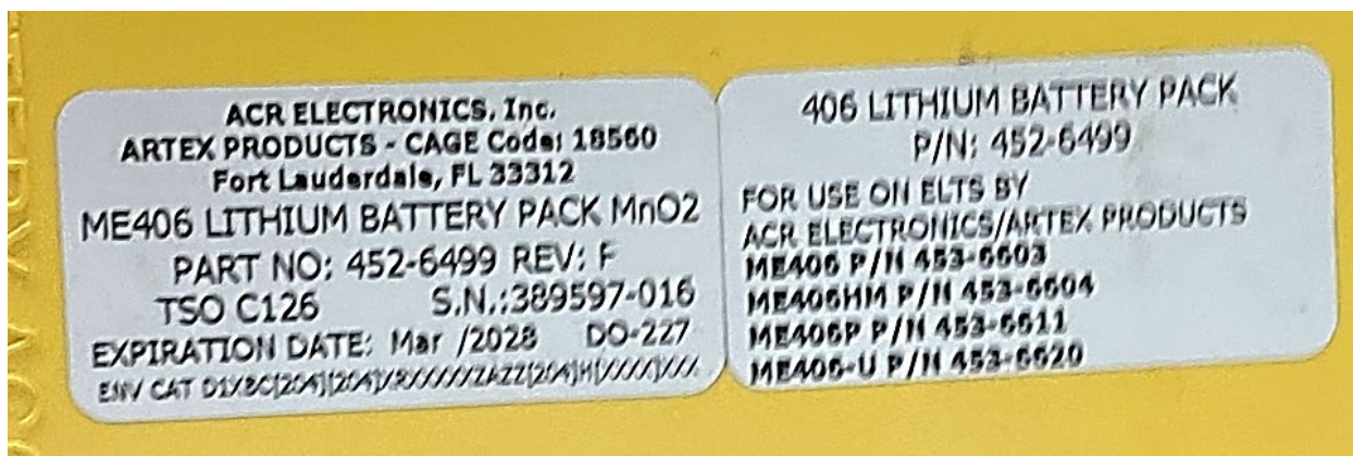
Figure 17. ELT battery information.
