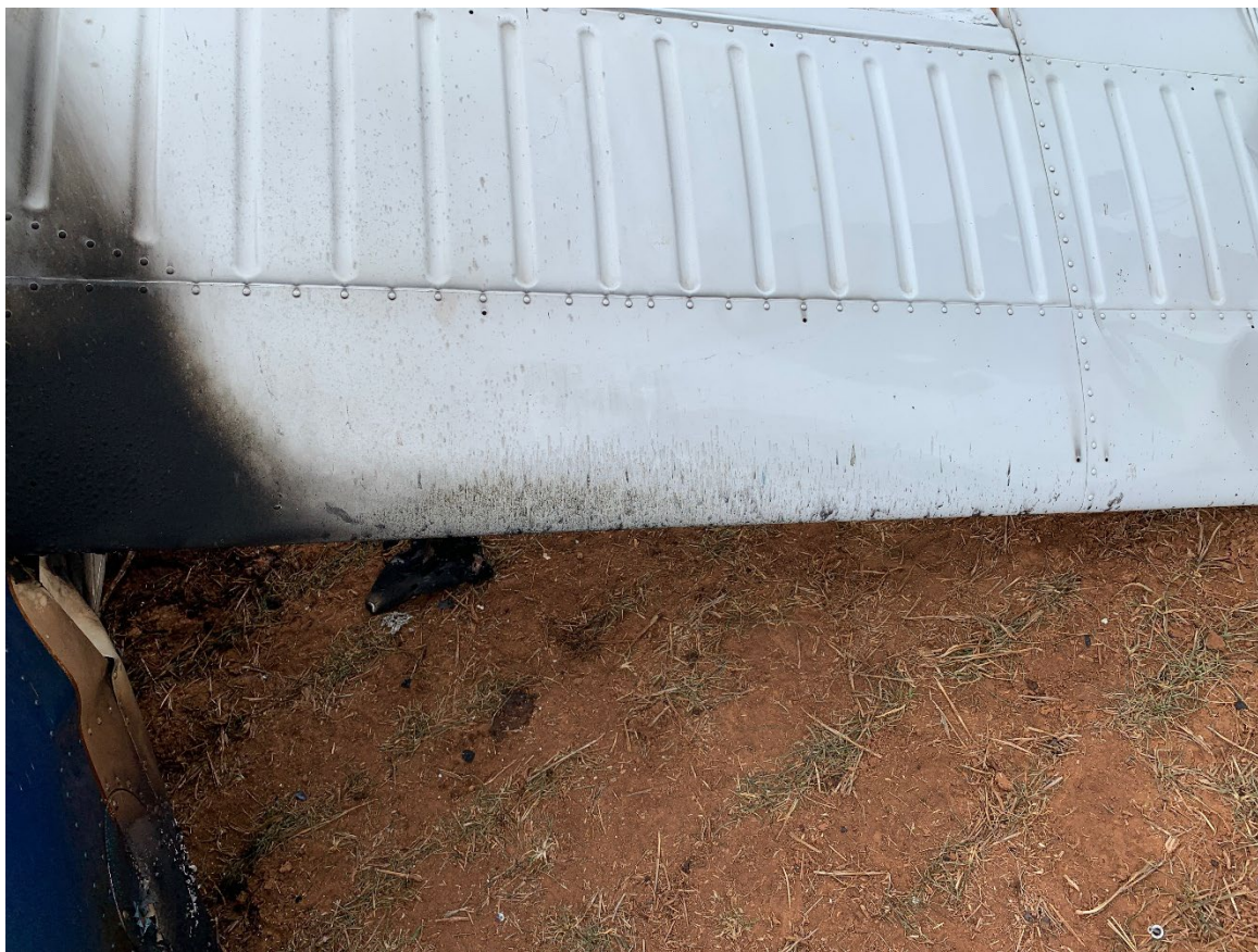
Photograph 7 - View of tail showing oil streaking and sooting (NTSB Photo)
