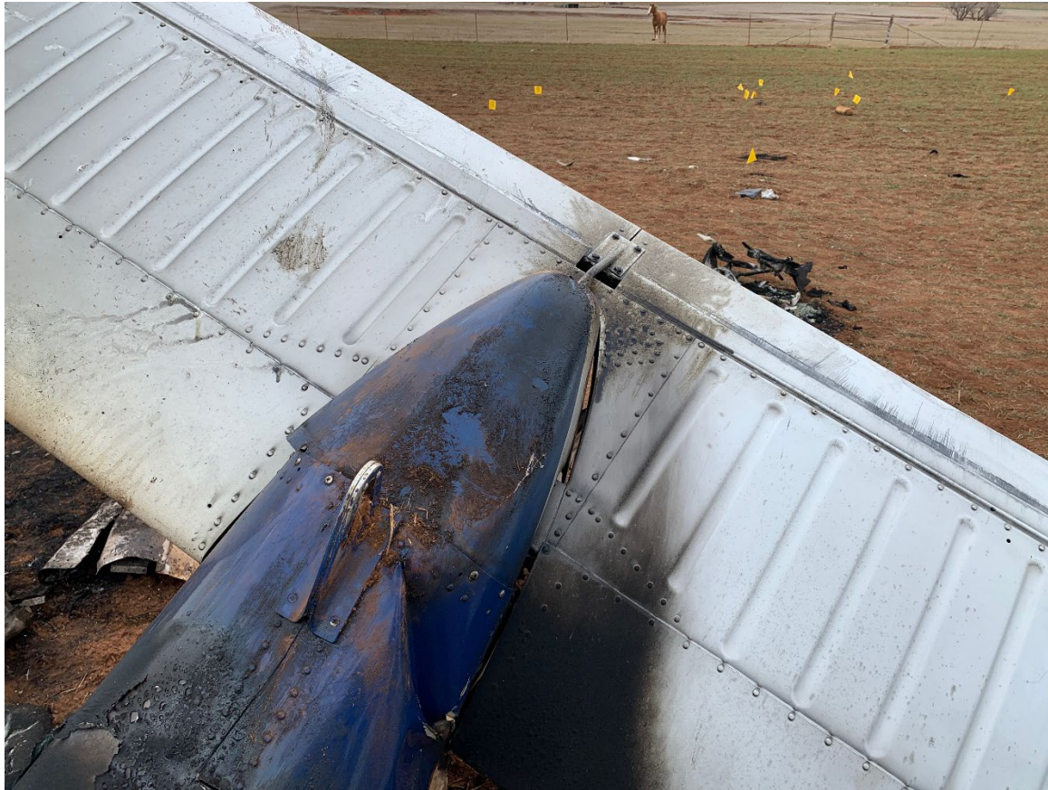
Photograph 6 - View of tail showing oil streaking and sooting (NTSB Photo)
