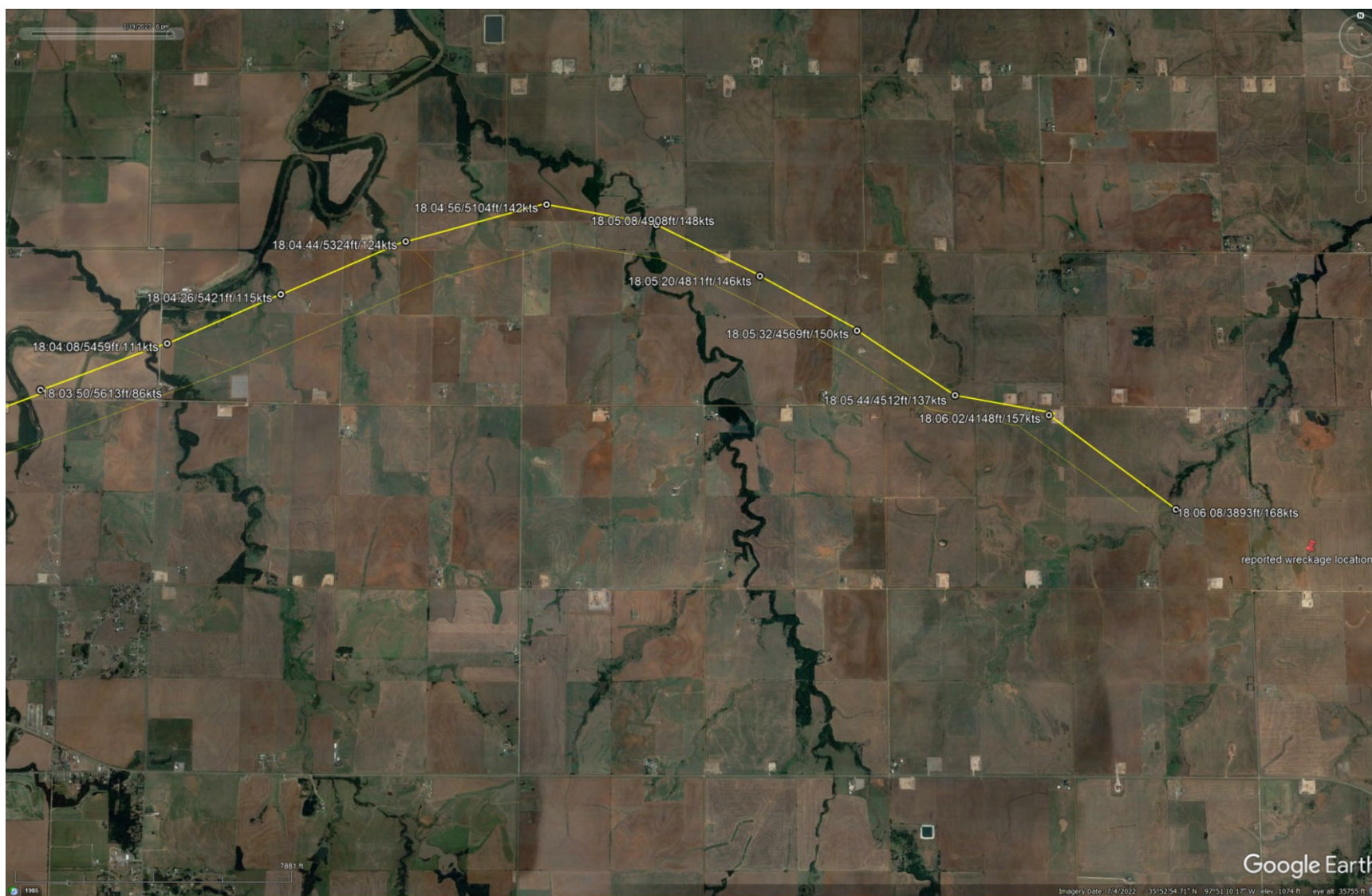
Figure 5. Google Earth overlay showing the end of the accident flight recorded on the JPI EDM-830 and the reported wreckage location.
